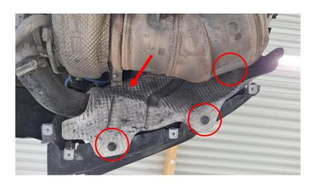
23. Remove the turbo inlet duct. 1x hose clamp, 1x Torx E10 (V-band), breather hose (right side only)
