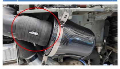
41. Strap the BOV hose and vacuum line (right side only) with the included zip-tie around fresh air duct. Make sure the zip-tie is placed where the aluminum joiner is.
