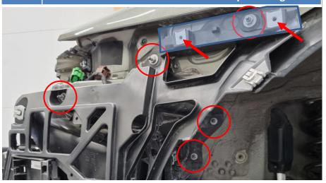
Now remove the entire plastic cage. On the right side you need to disconnect the vacuum line. Do this in the joint in between the plastic pipe and the rubber hose.
