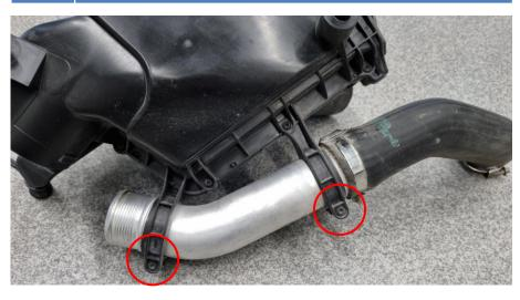
**31.** Reinstall the charge pipe in the car.
