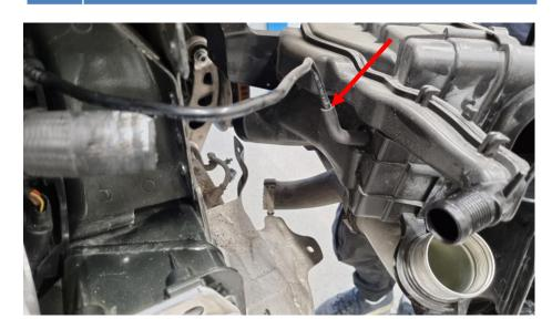
Remove the air filter box from the plastic cage.
