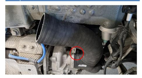
On the right side you need to disconnect the lower clips for the breather valve hose.
