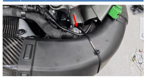
Reinstall the plastic air filter housing cage. Align the carbon fiber air filter housing so you have a few millimeters of clearance around the air filter housing. You may need to loosen the M6 Screw/nut for the large round bracket to adjust the rotation of the airbox. Finally install the included M6 washer and M6 Nut and then tighten all hose clamps. Reinstall all other parts in reverse order.
