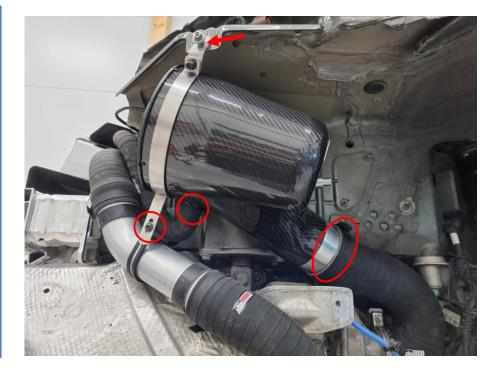
40. Install the plastic fresh air duct to the included square shaped silicone hose at the airbox inlet.
