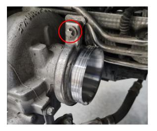
Install the included O-rings on the V-band hose adapters.
