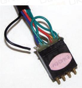
Broken or loose wires can result in lights not working properly
