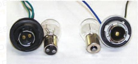
Two into one doesn't go - make sure the correct bulbs are fitted to the appropriate sockets
