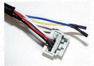
Wiring loom with spade terminals on connector block
