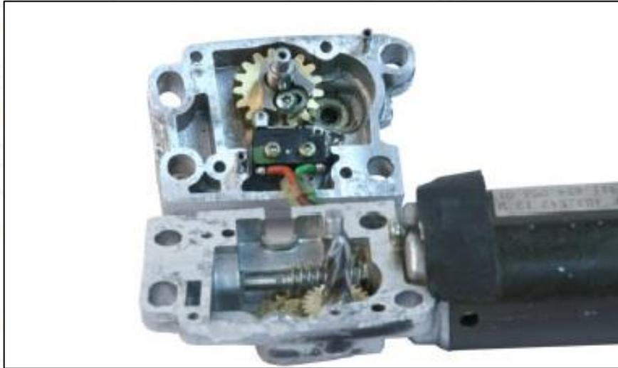
Install new drive gear / shaft assembly making sure it mates properly with motor pinion gear, taking care not to lose any of the distance shims under the old gear if present.
