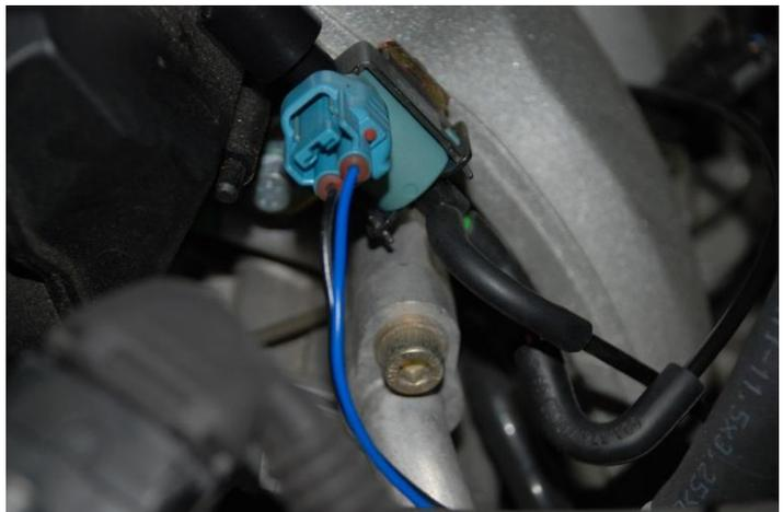
4. Follow the vacuum diagram to connect the solenoid valve to the intake manifold. NOTE: The white portion of the check valve MUST face the intake manifold. (DIAGRAM and PHOTO)
