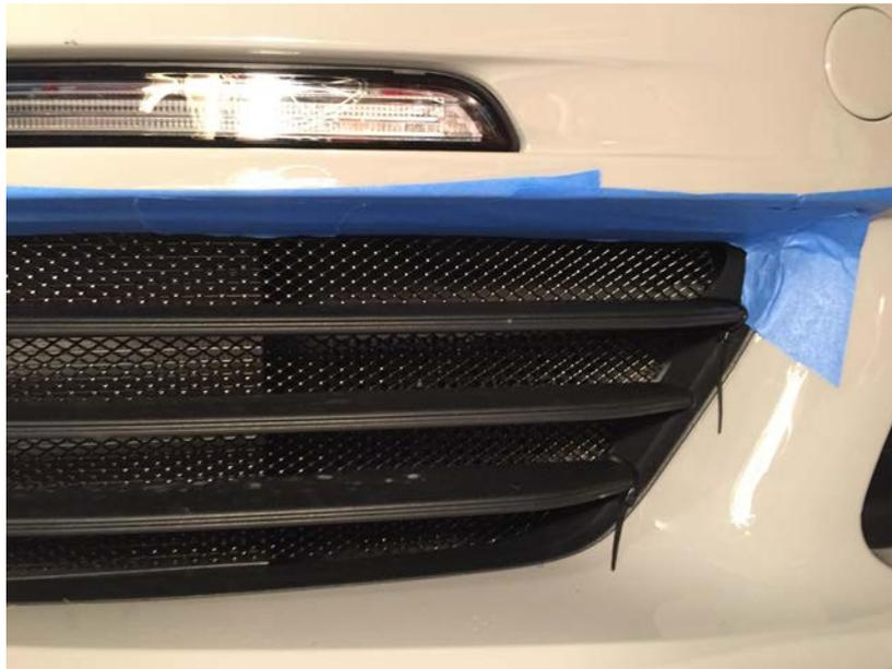
3. Clip off the ends of the cable ties. Complete!
