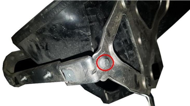
**28.** On both sides. Split the intercooler air guides by unclipping the 5 plastic fasteners that holds them together with a flat screw driver.
