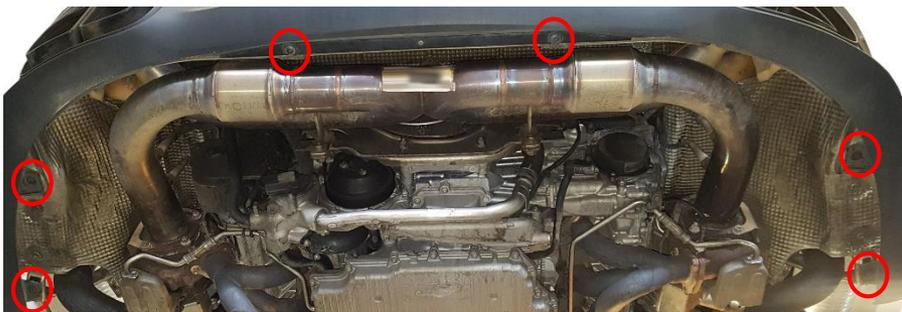
8. Remove 1pc Torx T30 screw in the top end of the bumper inside each wheel housing (hidden behind the wheel arch plastic).
