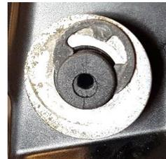
**27.** On both sides. Remove 3x Hex 10mm screws and gently split the intercooler console. Remove the intercooler and air guides from the console. Make sure the rubber grommets are left in place in the console.
