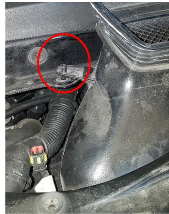
17. Now remove the wing motor plate.
