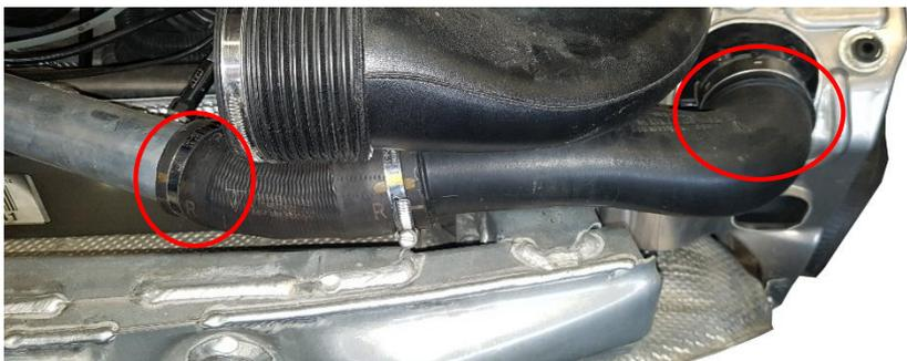
20. Disconnect the bypass valve vacuum line hoses on both sides.
