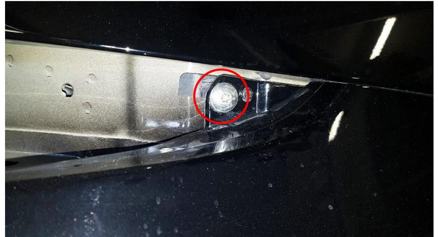
7. Remove 6x Torx T30 screws along the bottom of the bumper.
