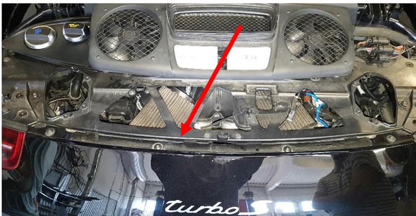
18. Remove 2x hose clamps, left side breather valve, right side solenoid valve and vacuum line. Then remove the air filter box.
