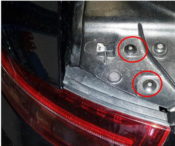
6. Remove 1x Torx T30 screw hidden behind rear light on both sides.
