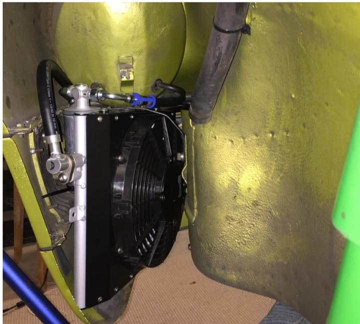
The condenser assembly has been test fitted on an 1982 SC so we know it fits this model. It will also fit single battery 911s prior to 1969 as the space here is empty.
