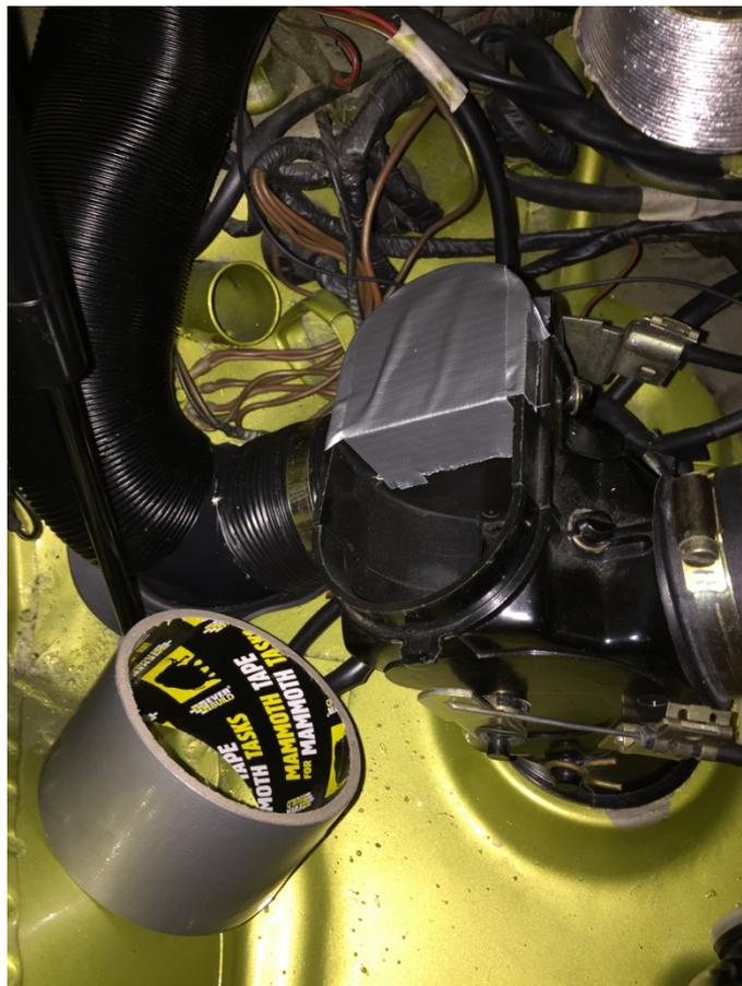
Blocking off the rear of the blend valve duct. Do this for both sides. Don't worry, you will still get warm air to the screen. You can also see the SC type side vent tube which is part of the bodywork. Connect 40mm tubing here.
