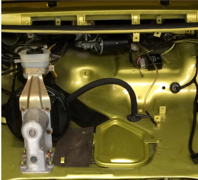
With old blower removed, identify holes for cabin wiring and wire sense lines to high power accessory switches.
