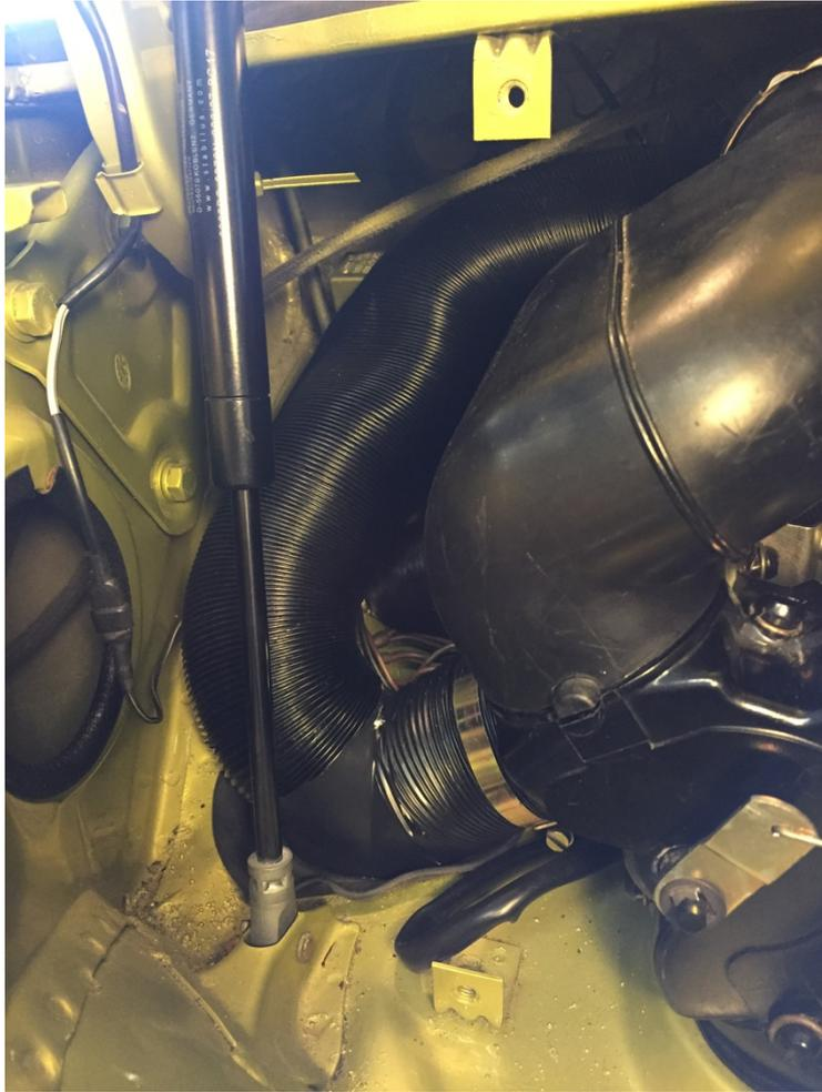
'T' piece in place (bottom of picture) with branch running to inlet of new blower.
