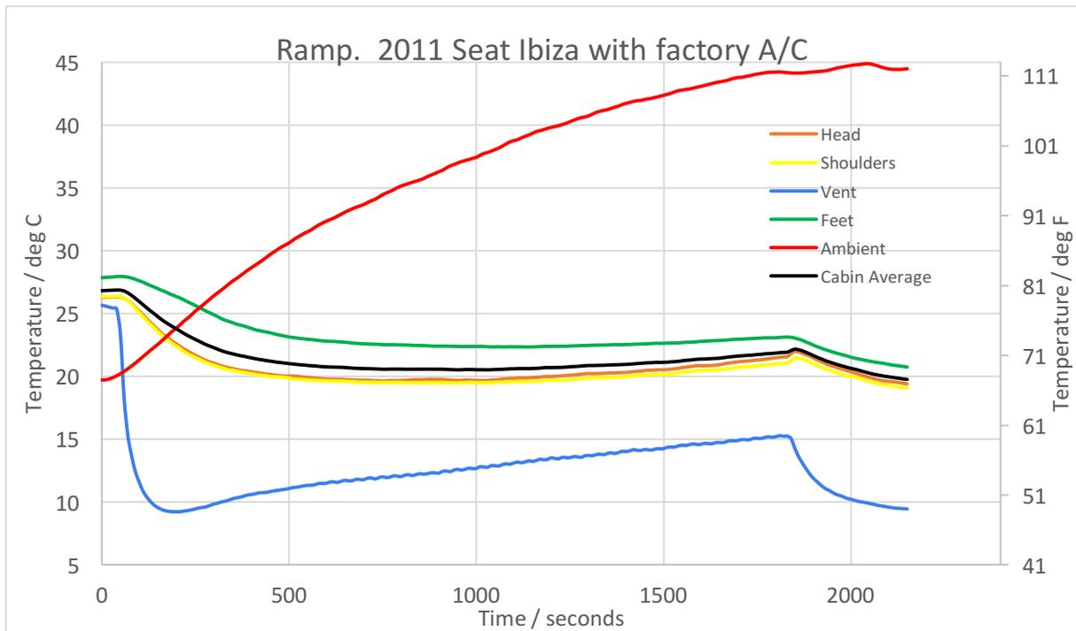
The soak test was started after leaving the doors open to bring the cabin temperature up towards ambient. Excellent as expected. Strong blower fan, good recirc and insulation.
