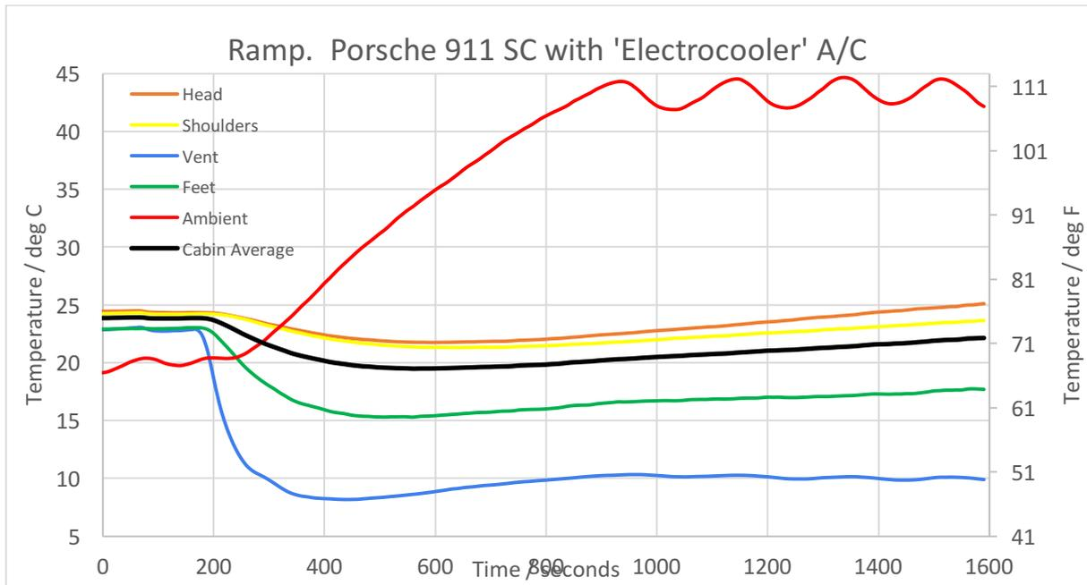
Good vent temperatures. Needs more airflow to reduce cabin temperature.
