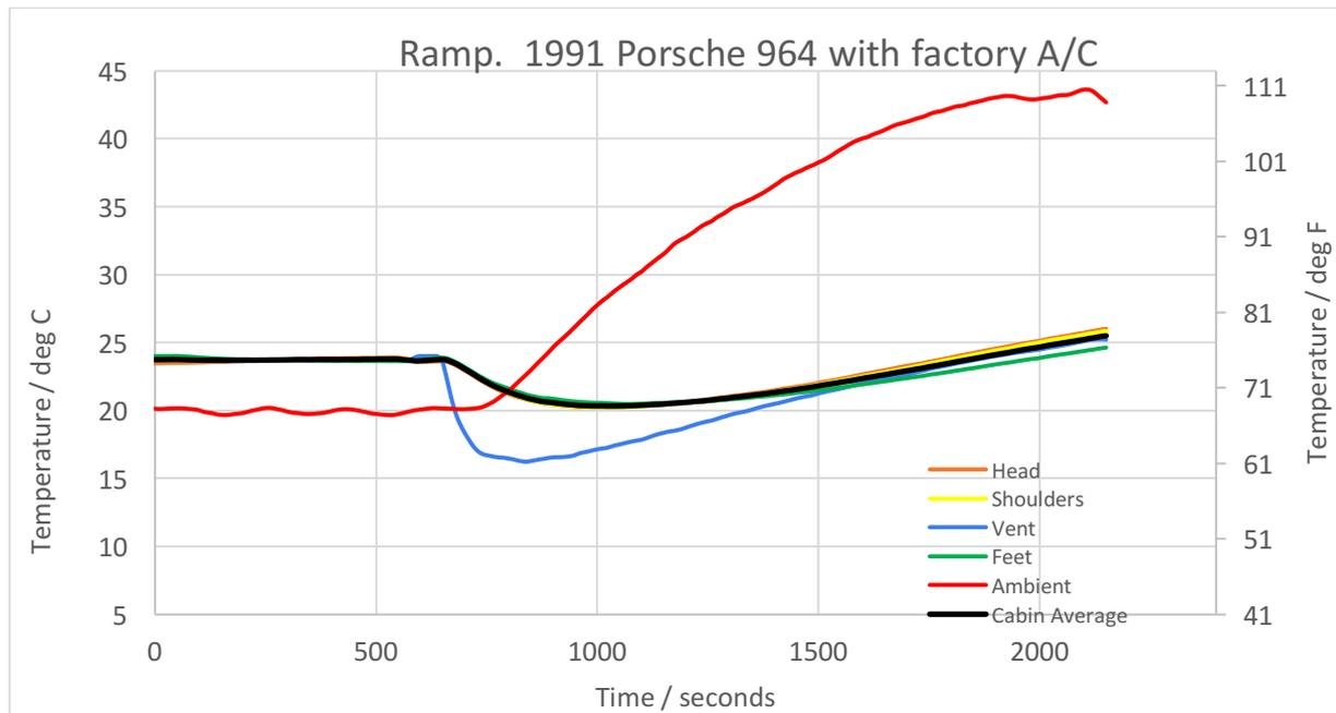
Heat soak test suffers because of poor vent temperature, although fan is better than 911.
