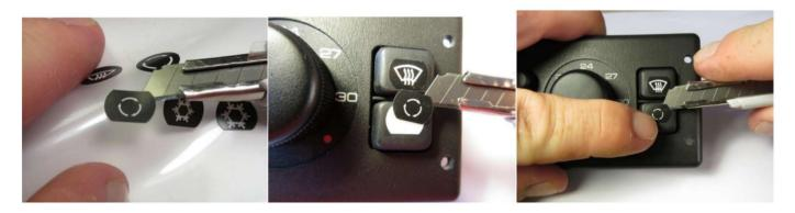
The stickers are produced with a silk matte finish, but they may appear a bit shinier than rest of the surface of the switches. To obtain a more matte finish, you can use 1000-Grit sand paper and very carefully sand the surface of the stickers. Be careful not to sand too deep and damage the laminated coating.
