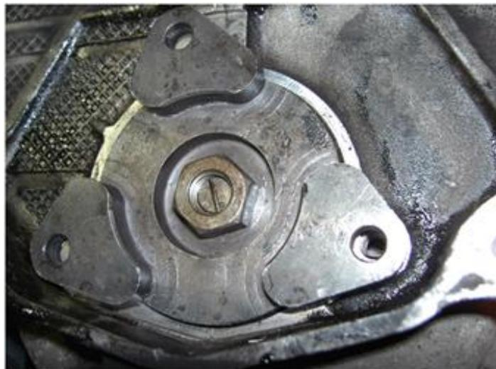
With the new flange centered, carefully tap it in with a brass or rubber mallet, being careful not to hit the bearing's center shaft
