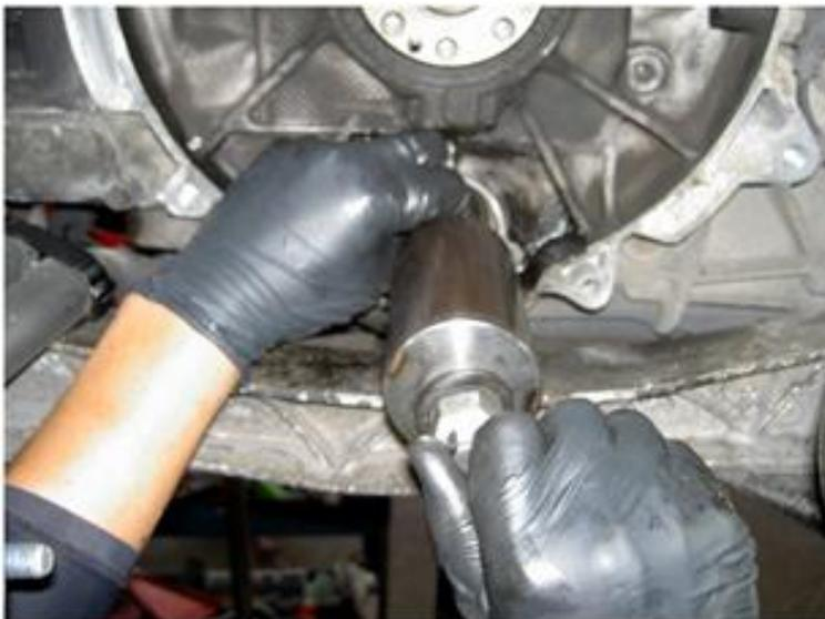
... and thread the center bolt onto the IMS bearing shaft. Tighten it by hand. Tighten the tool's center nut by hand all the way down making sure that the IMS Removal Tool is completely seated at the base of the engine block.
