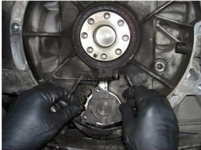
Using a flat screwdriver turn it Counter Clockwise (ccw) to get the first two or three threads of the center shaft exposed
