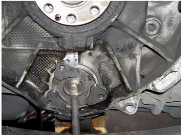
Once the first couple of threads are out, insert the center nut and tighten by hand.
