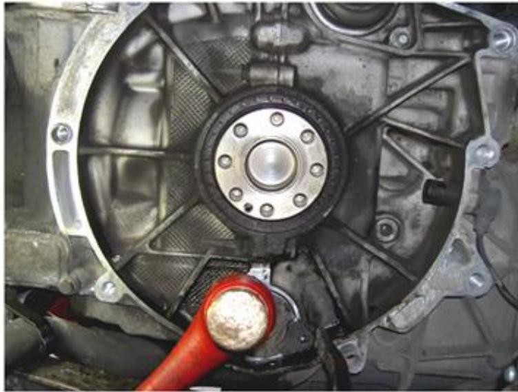
a bead of thread lock onto the three clean flange bolts
