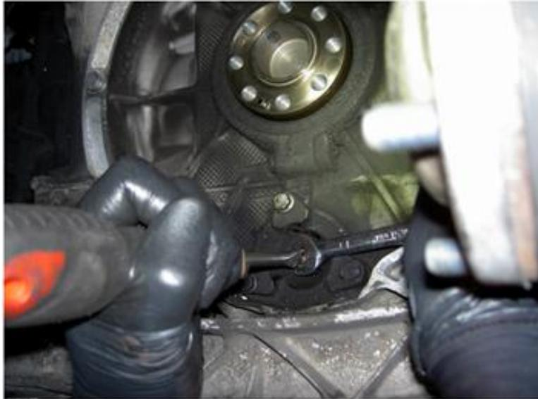
Remove the three flange support bolts.
