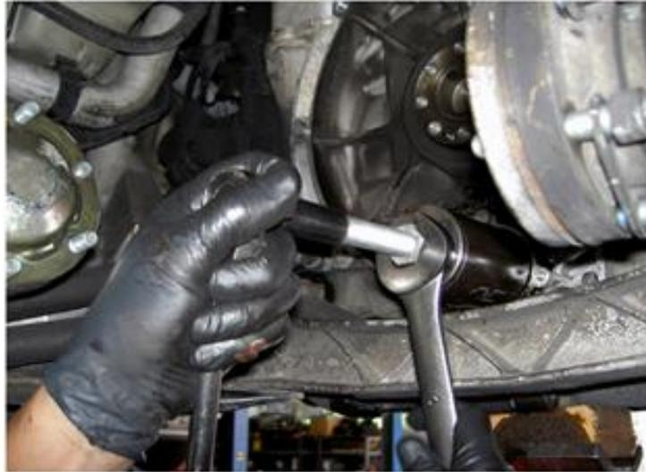
You might hear a loud “pop” which is normal. Continue tightening until the bearing comes loose and can be pulled out completely.
