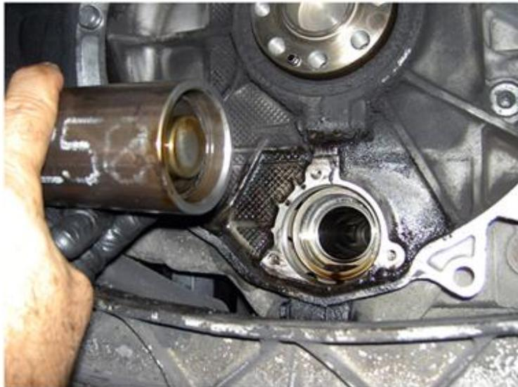
Thoroughly clean the bearing seat area and remove any debris, engine oil, etc.
