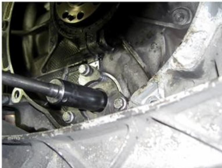
If you need to replace the Rear Main Seal (RMS) this is the time. Use a strong metal pick to pull out the damaged seal and install the new one in place. Follow the RMS' installation procedures (depending on the manufacturer).
