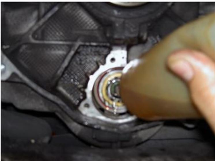
Smear a bit of grease onto the new flange's O-ring to allow for an easier installation
