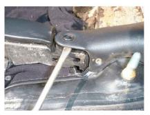
Remove the rubber seals on both sides of your top by taking out the screws in the rubber apertures (picture 2A). Now remove the 2 steel guides left and right (picture 2B). Use a metric spanner (M13) to remove the top guide pins (picture 2C). You roof skin can now be removed.
