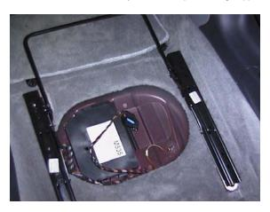
Step 4. Attach racing seat to sliders per manufacturer's specs.
