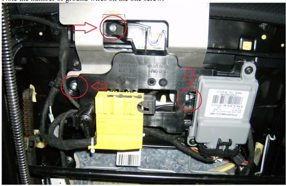
Step 5. Seats with power sliders only: A single wire tie down must be moved to create clearance for the R-2050, as pictured:
