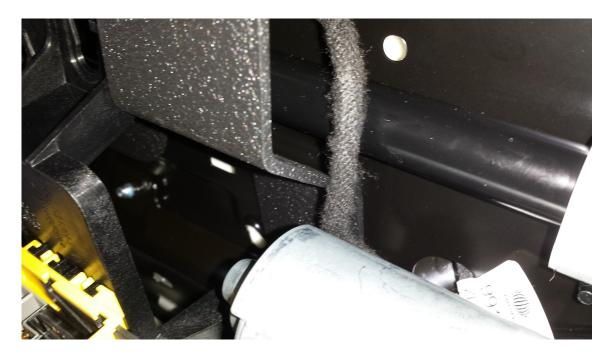
Step 6. Position the fire extinguisher mount under the bracket. Use the factory supplied bolts and washers. Be sure to reattach the ground wires.
