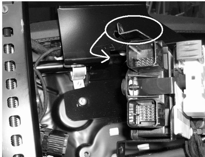
Step 8. Place spacer under front of bracket. Install 6mm X 70mm bolt with washer through spacer and module leg. ( Use a small Allen wrench or awl to align the brackets and the insert bolt). Note: Do not over tighten this bolt.
