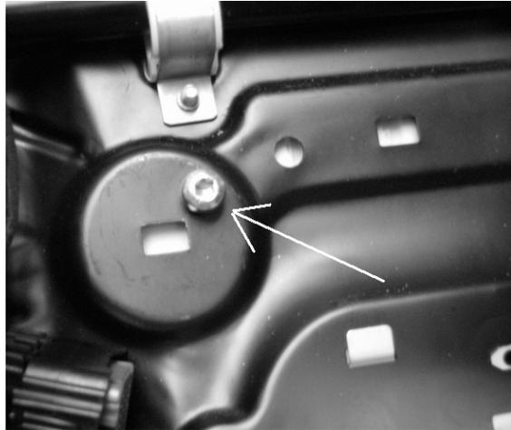
Step 6. Position the fire extinguisher bracket. Install the screw under the module first (the one you just tapped). Align the opposite hole then tighten screw.
