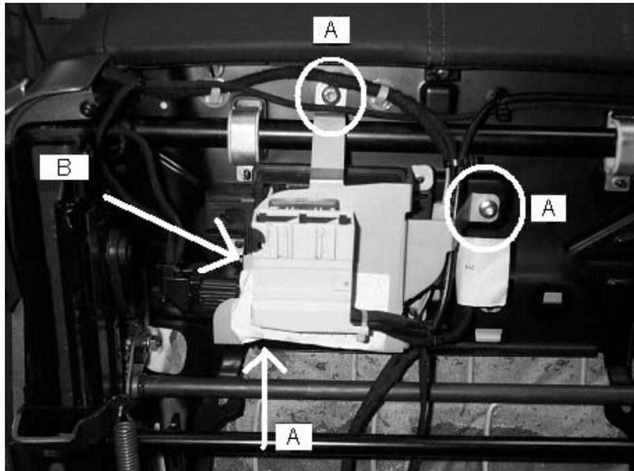
Step 5. Tilt the module to access the mounting hole. Use one of the removed self tapping screws to thread this hole.( At Location B)
