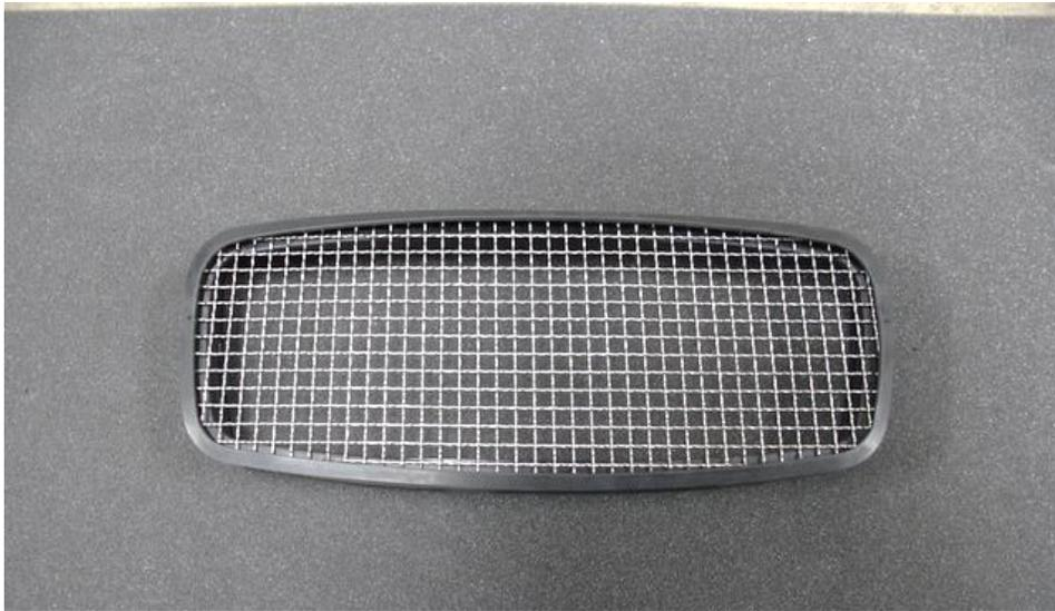
17. Insert the mesh into the rubber surround at the base. The Eventuri logo should be at the top (not shown here). Back of the rubber surround shown above.
