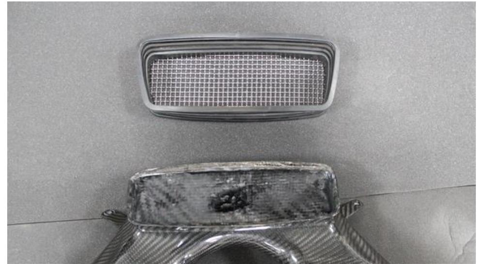
18. Take the carbon duct and now push the rubber surround with mesh into the top of the new duct.
