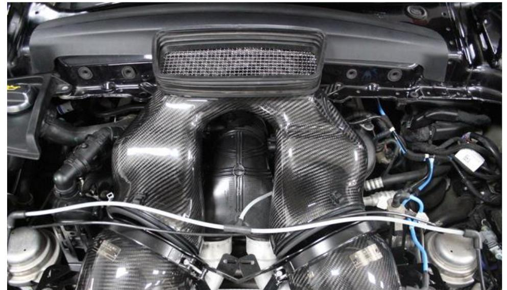
20. Now place the duct on top of the filter housings. We will now line up the housings to the duct.
