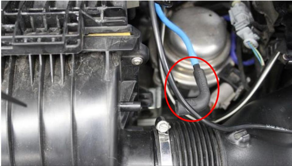
5. Remove the Vacuum connector from the right side of the airbox. It will pull out.
