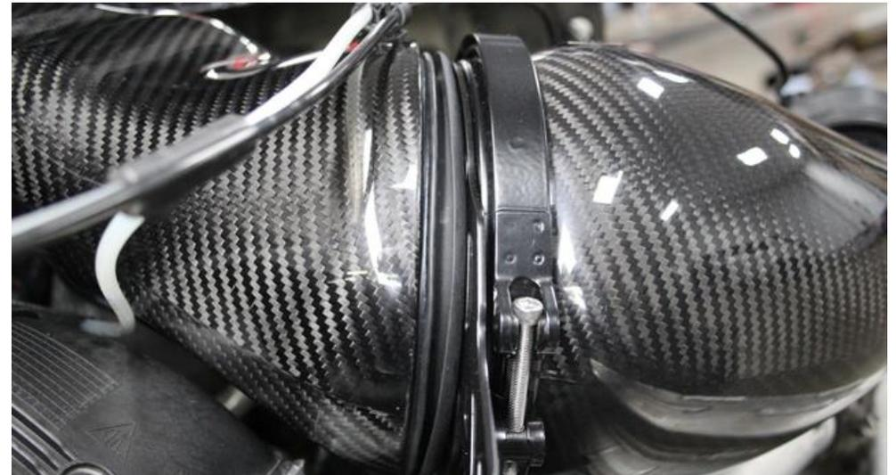
26. Once fully sealed as shown, tighten the large clamp around the housing.
