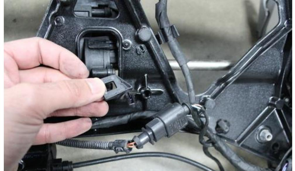
34. With the connector unclipped, remove the bracket for the connector from the frame.
