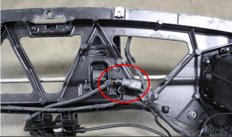
33. For extra clearance – unclip the connector from the underside of the metal frame which holds the spoiler motors.
