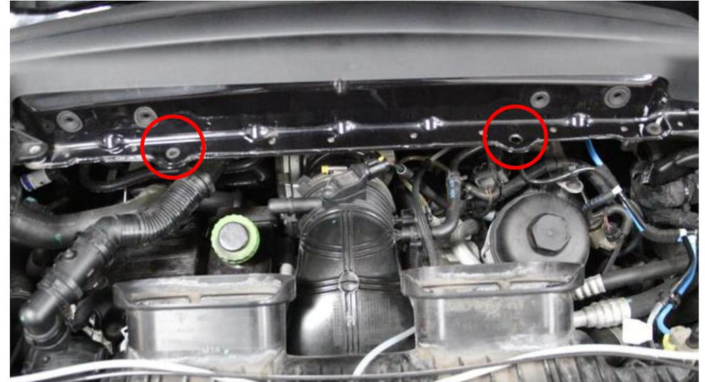
6. Remove the intake duct by simply pulling it upwards. It is held in place with rubber grommets which are circled above.
