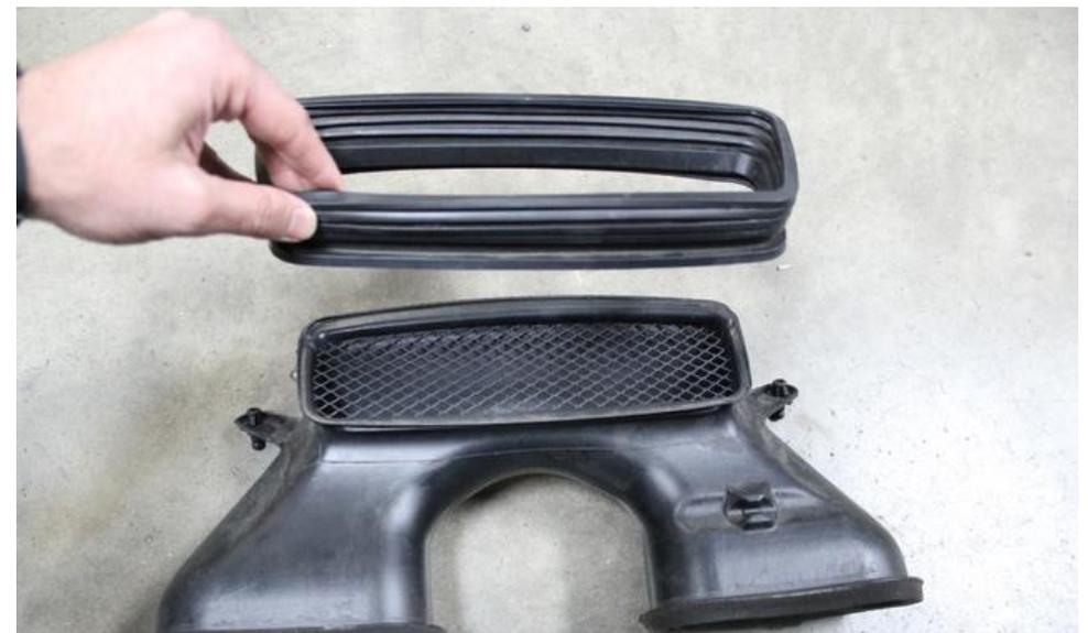
8. Remove the rubber surround from the top of the duct. We will use this later.
