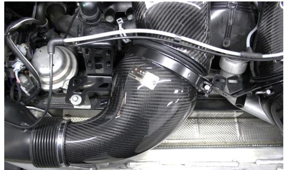
28. Repeat this process for the other side. Once lined up, secure the large filter clamp and the hose clamp around the stock inlet pipe.
