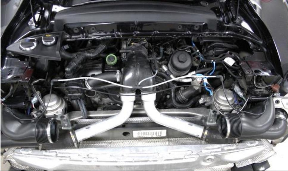
9. Loosen the 2 hose clamps on each side of the airbox at the outlets and then the airbox can be removed from the engine bay.
