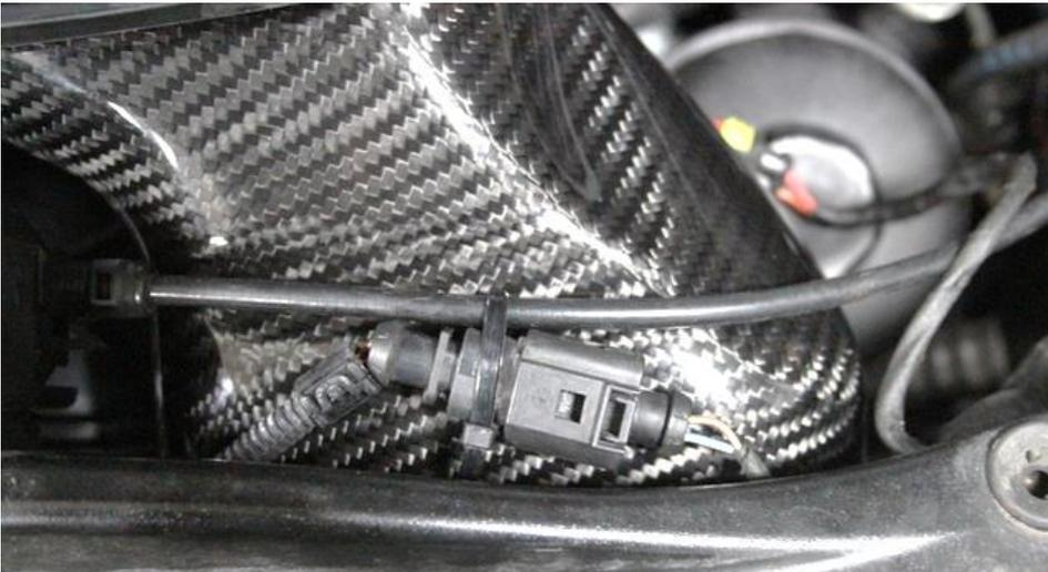
35. When this frame is back into position – secure the connector to the bootlid release cable with the supplied cable tie. This allows the required clearance between the duct and the frame.
