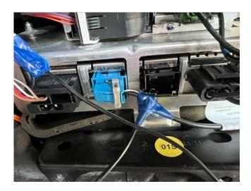
**Please note** that the OEM TV module is only FO bypassed, it must be still connected to the power cable.
