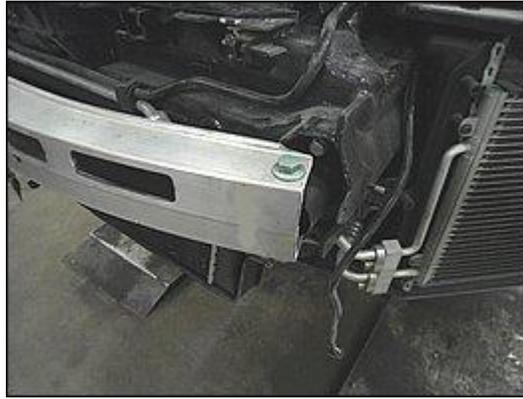
You may also need to bring the front bumper beam forward slightly by using a packer made from metal and longer bolts
