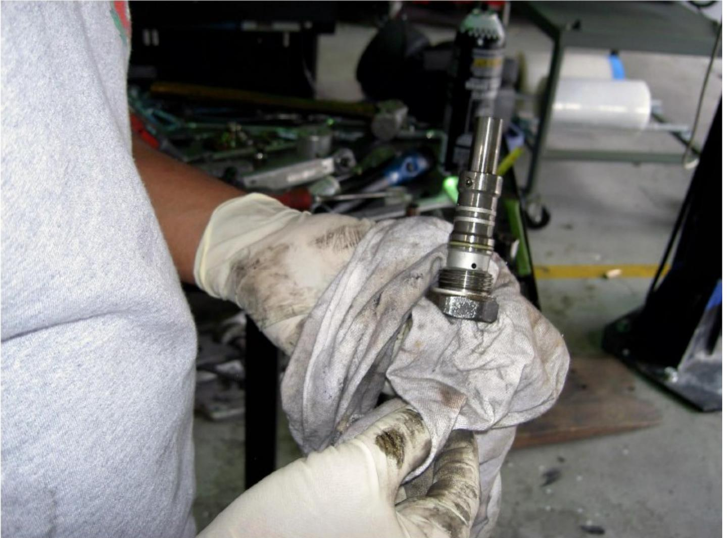
Insert and tighten the chain tensioner.
