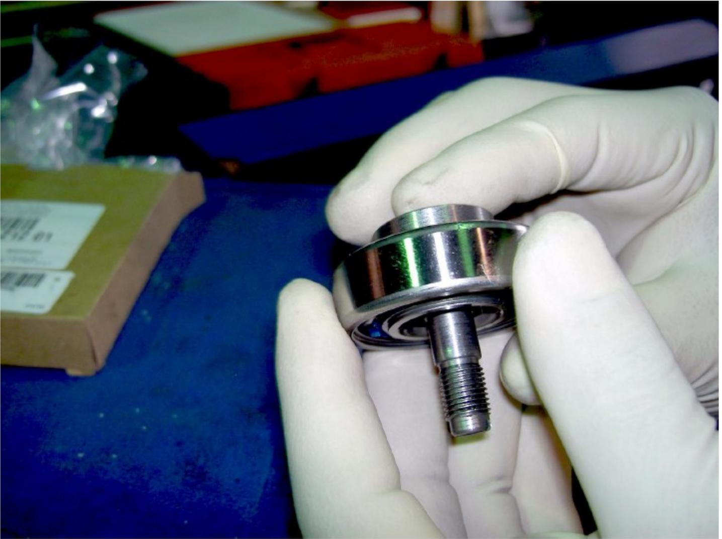
Place the bearing with the shaft in place over a socket of the correct size which can support the inner race of the bearing and lightly tap the end of the shaft completely onto the bearing's inner race.
