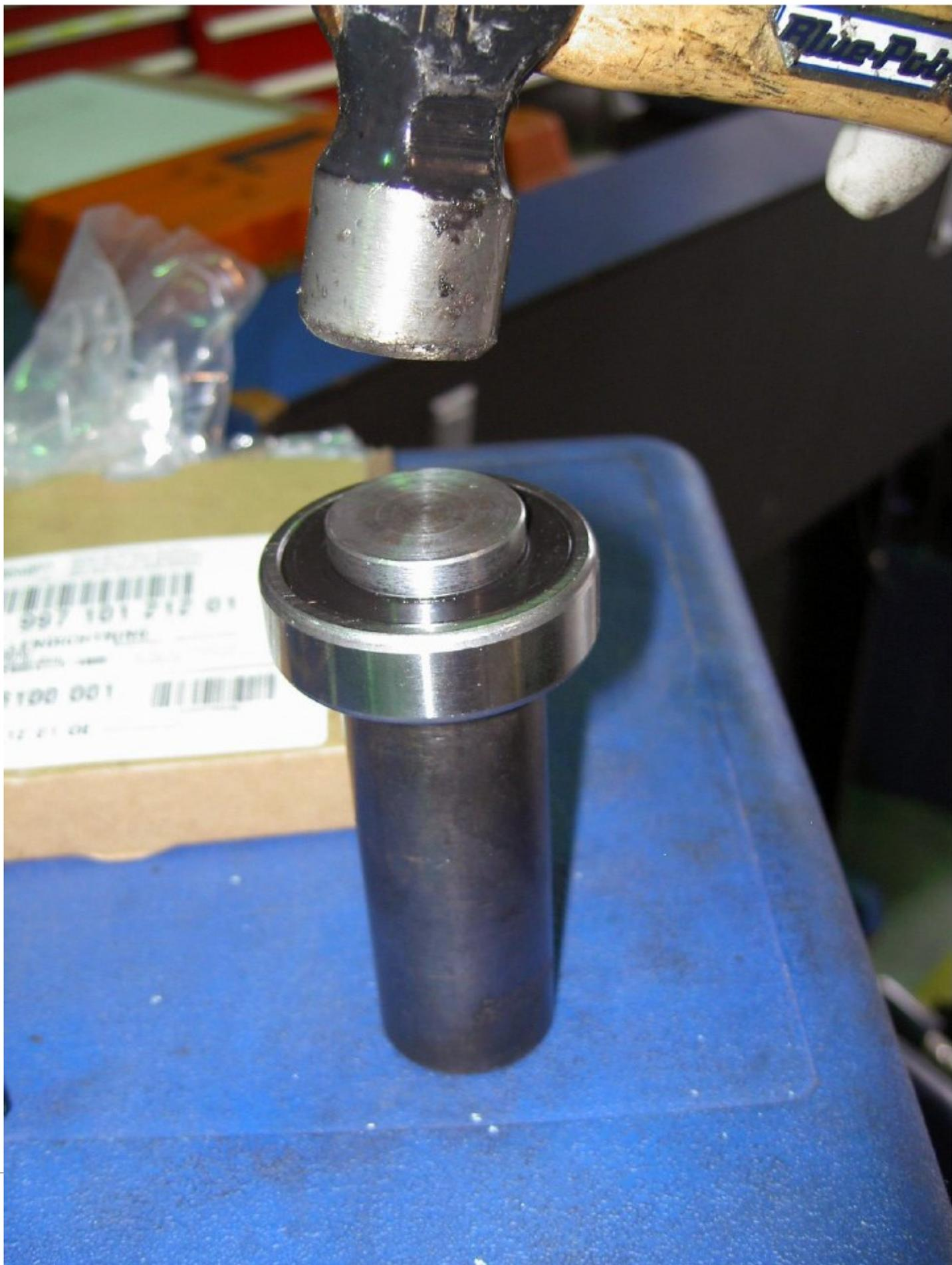
Place the assembly into the bearing insertion tool.
