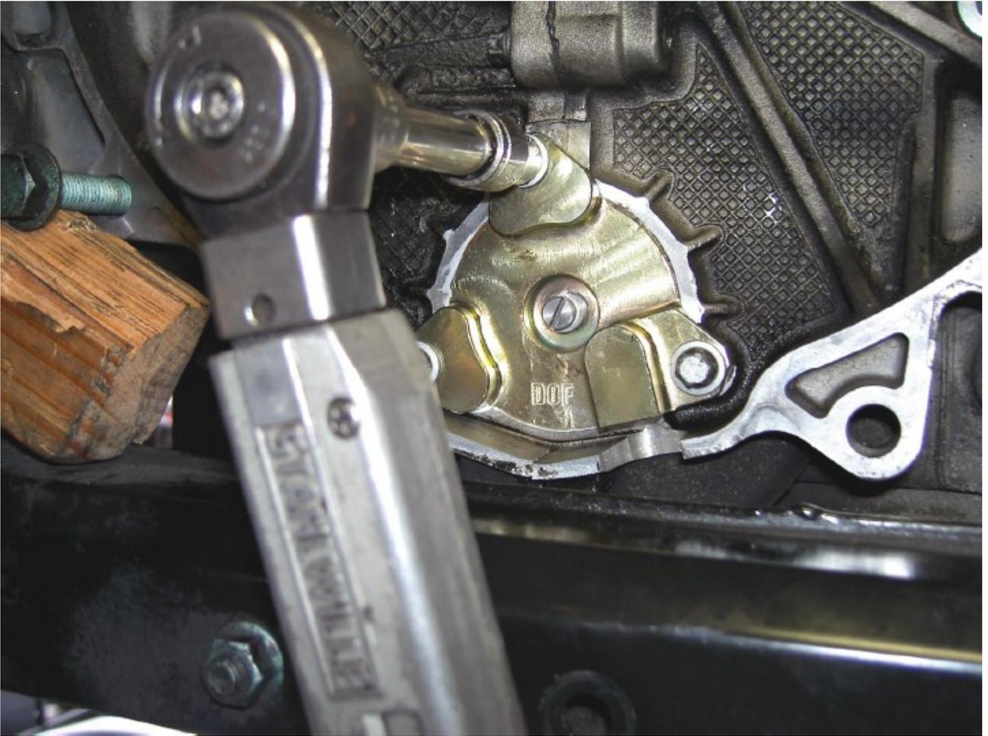
Put a bit of thread locker (supplied) onto the threads of the new bearing support flange nut (supplied) and thread in place by hand.
