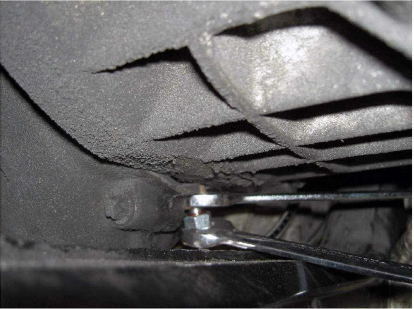
On Boxsters replace the earlier removed engine safety cable to the engine support yolk and tighten. In the case of the Carrera, replace the rear sway bar and tighten.
