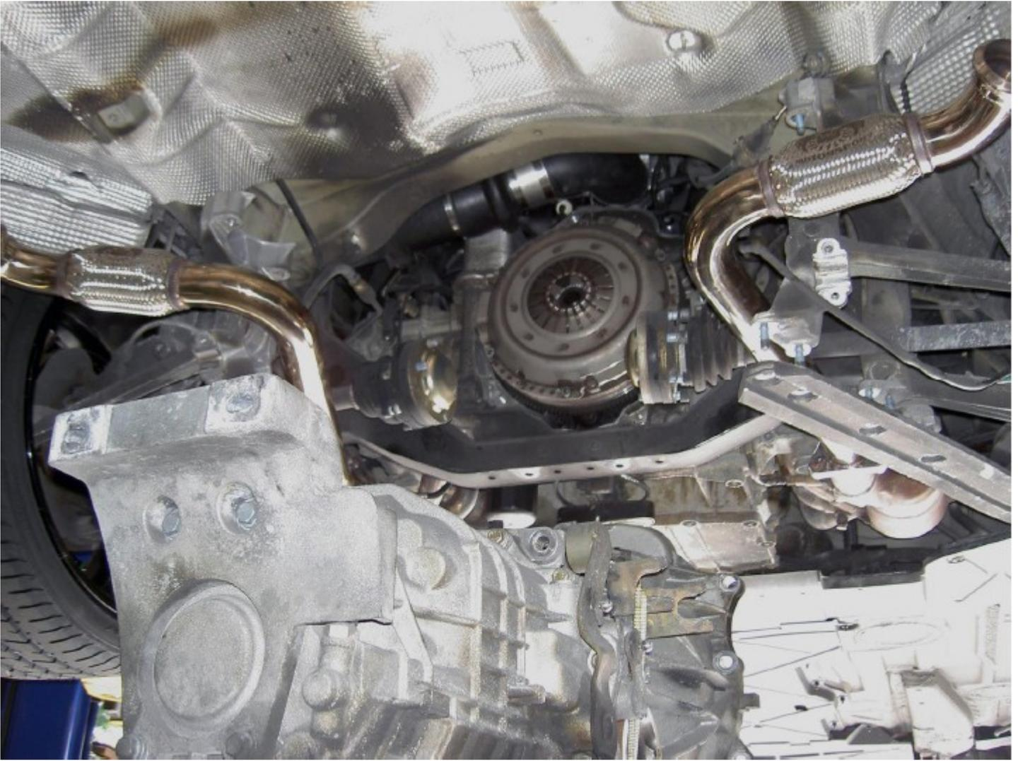
Remove the clutch assembly (or torque converter).
