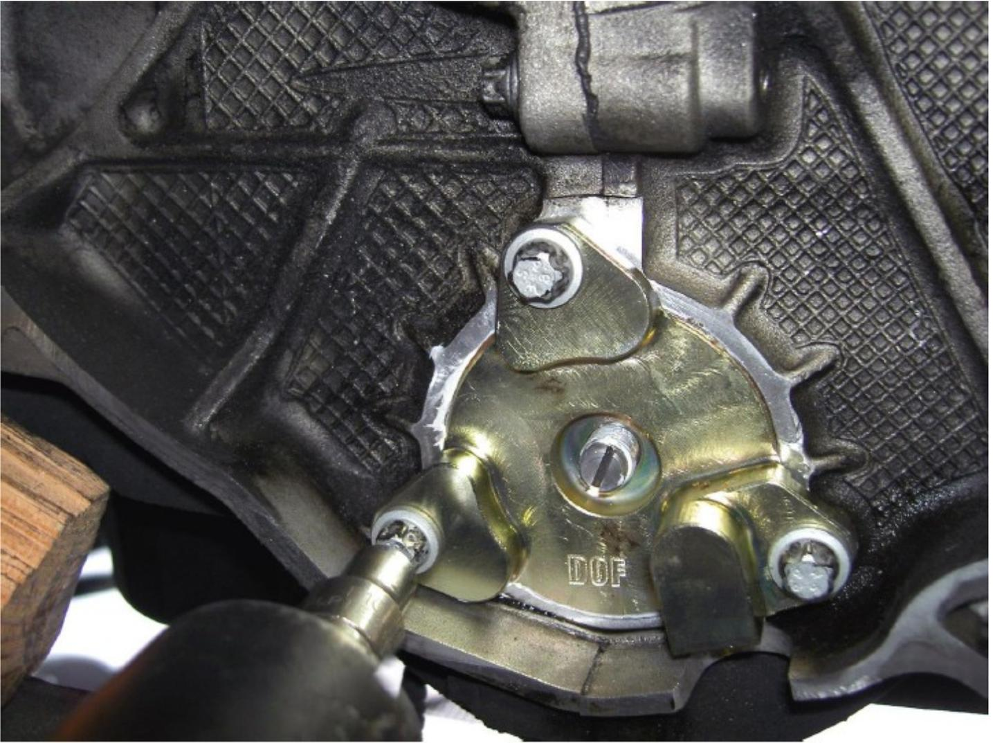
Once all three bolts are completely screwed in and the flange has been seated, tighten to a torque of 10 Nm (7.5 lb-ft or 88.5 lb-in).
