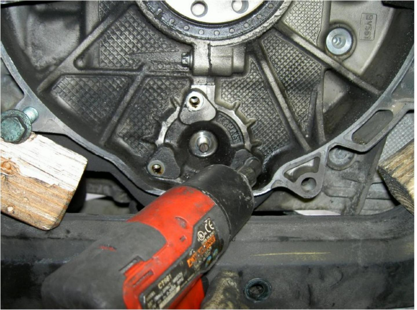
Using a couple of flat-bladed pry bars or strong screwdrivers slowly and carefully pry out the existing bearing flange.
