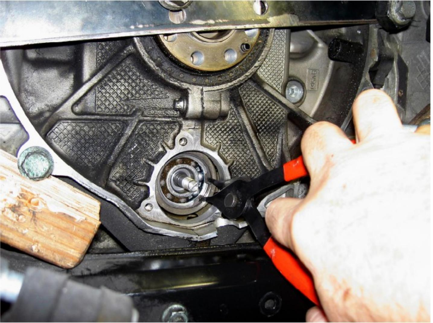
Screw the center bolt from the bearing removal tool onto the bearing's support shaft and tighten by hand.
