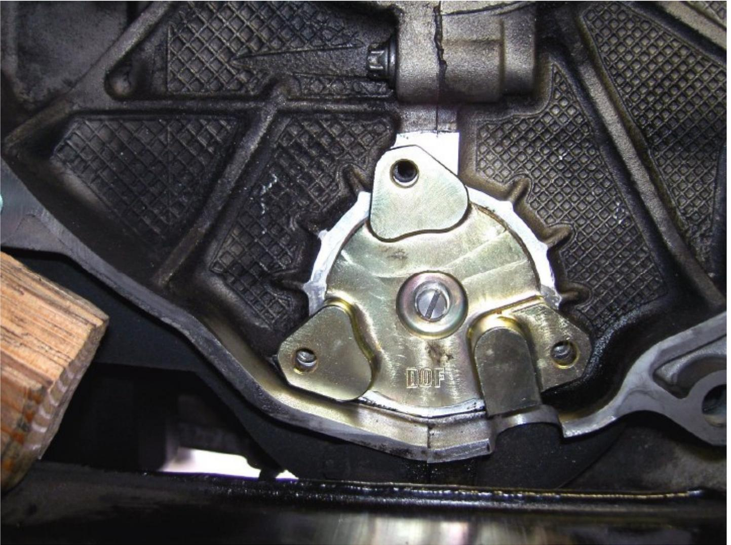
Check the clearance for the DOF/Oil line screw-in adapter on the bell housing cut-out that you made before. Adjust the clearance if necessary with a file.
