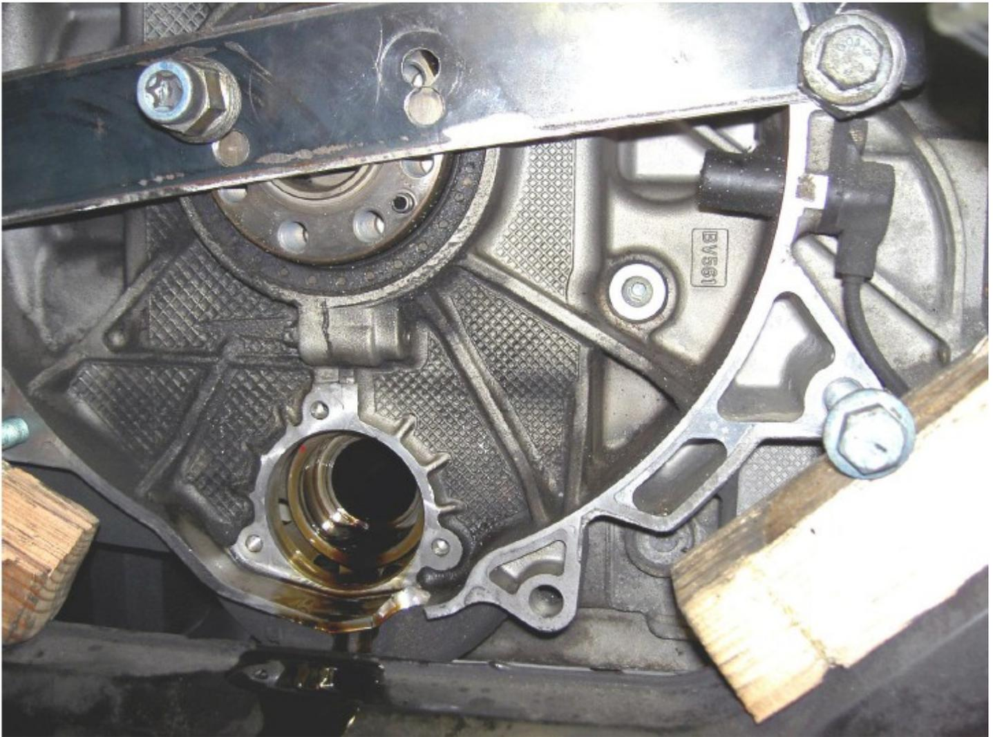
Clean out the open end of the IMS. Leave a thin film of oil or grease so that the new bearing slides in easier.
