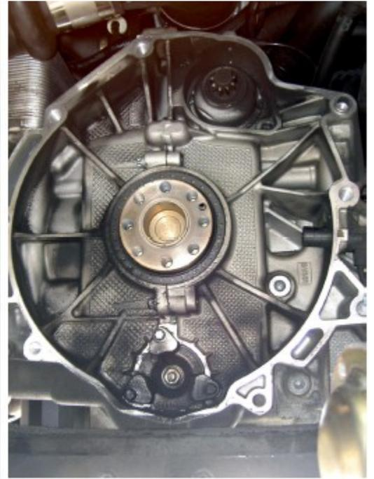
Inspect the rear main seal (RMS) and determine if it will be replaced due to leaks. If replacement is needed, do so after the DOF installation.
