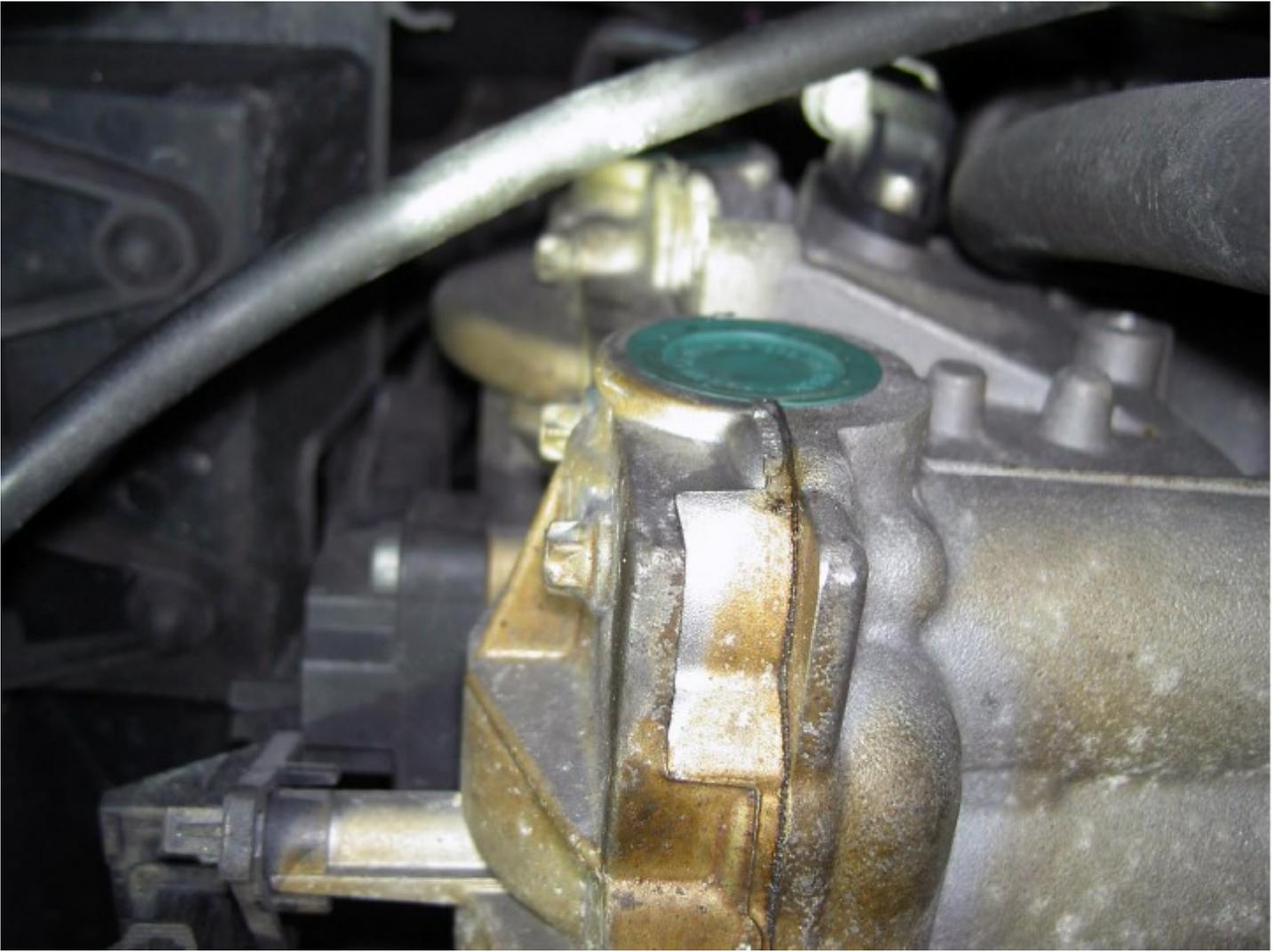
From the top of the engine thread the angled end of the high pressure oil line down to the DOF and thread into place.
