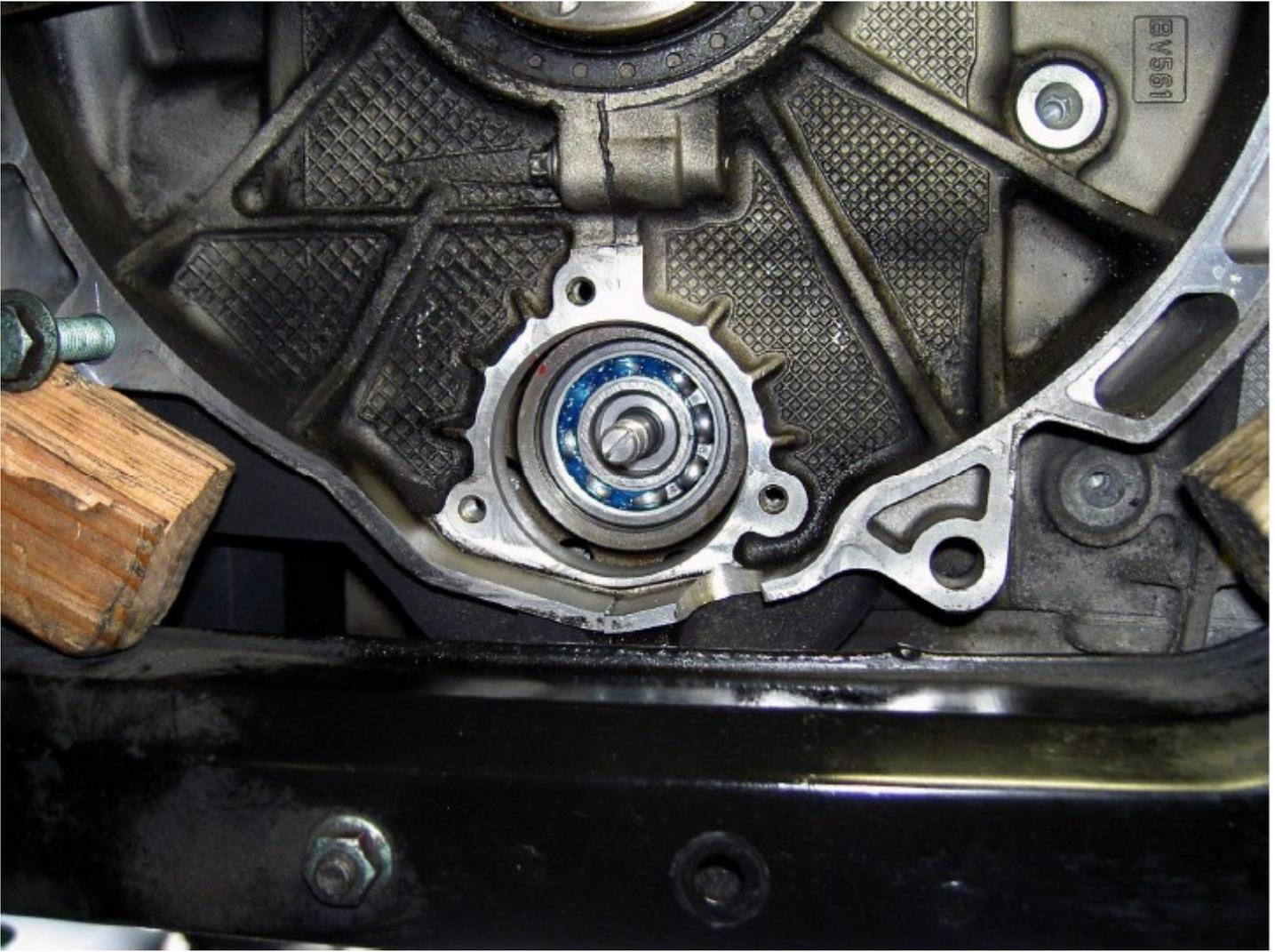
Using the proper C-clip pliers insert the new retaining clip (supplied).
