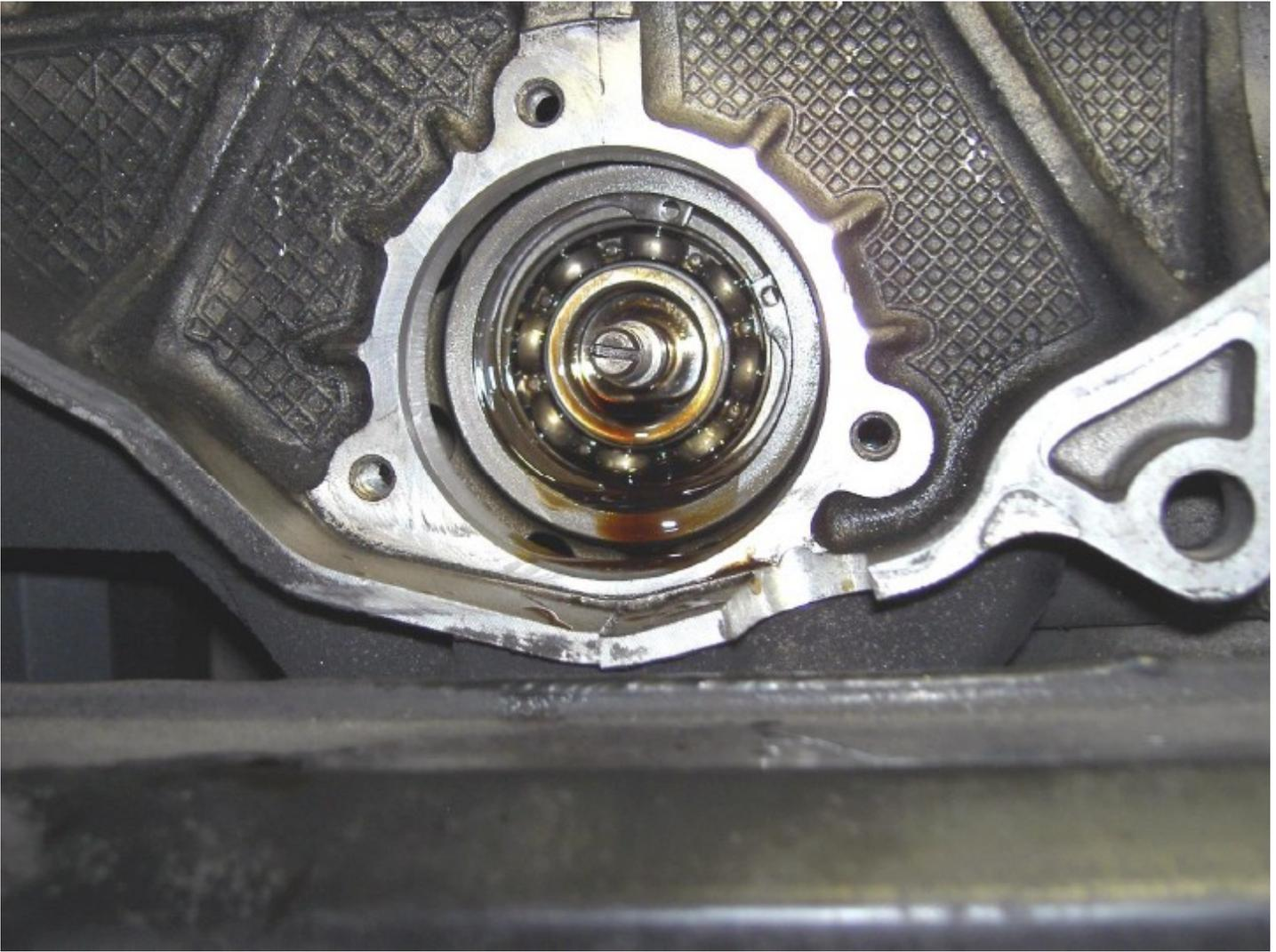
If the IMS bearing is to be replaced, remove the retaining C-clip.
