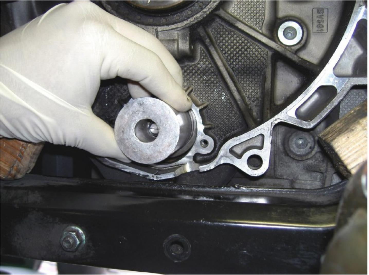
Tap the end of the insertion tool until the bearing is seated completely. You will hear a “solid” change in sound when the bearing has reached the engine block.
