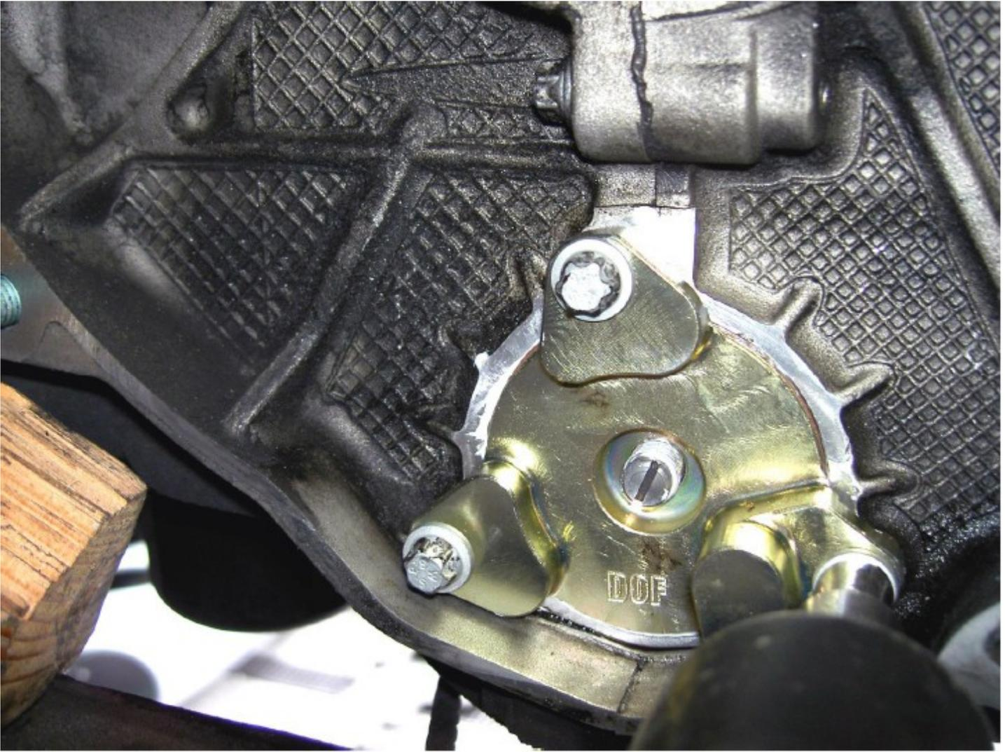
Tighten each bolt only a few turns at a time and move to the next one. This assures that the flange gets inserted correctly.
