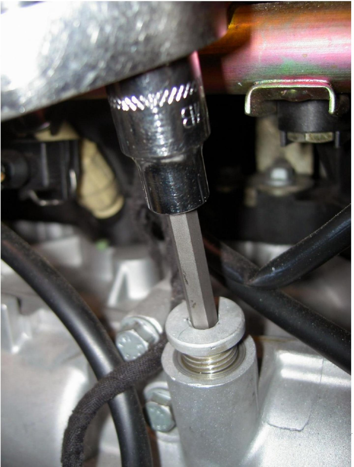
Place the copper crush ring onto the 14 mm end of the hose adapter. Put a couple of drops of thread locker (supplied) and thread onto the engine. Torque to 15 Nm (11 lb-ft or 132 lb-in).
