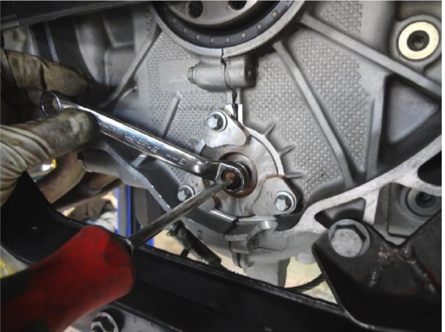
Remove the three flange support bolts.
