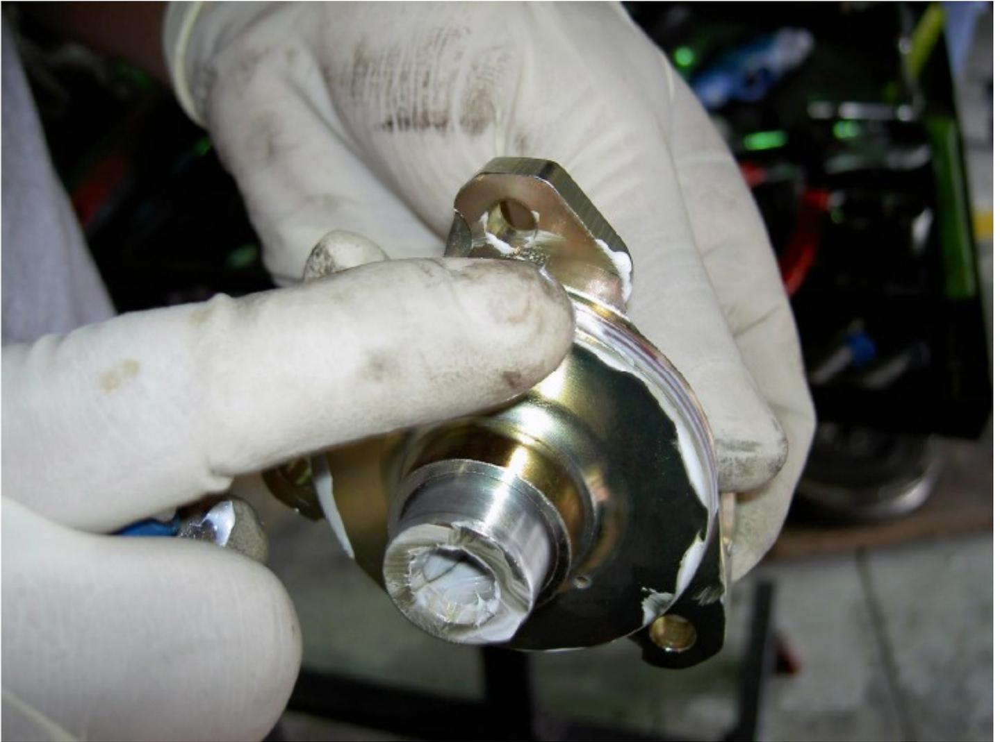
Place the new DOF flange with spacer ring in place onto the bearing support shaft.
