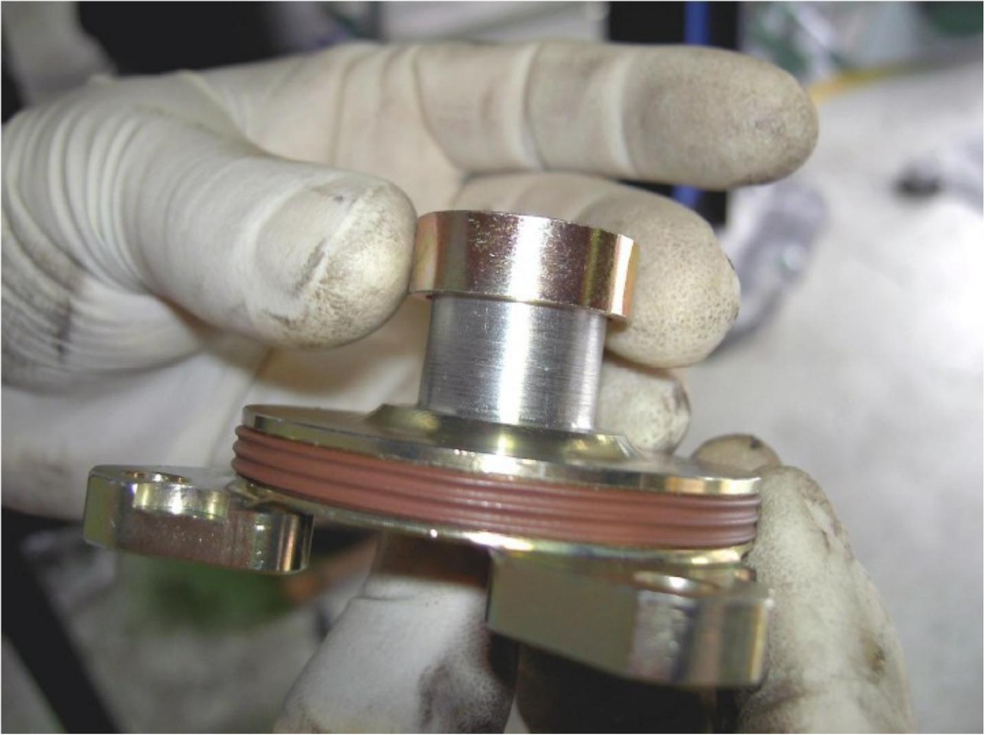
Smear a bit of high-quality white lithium grease on the inside of the DOF shaft and on the outside red sealing ring.
