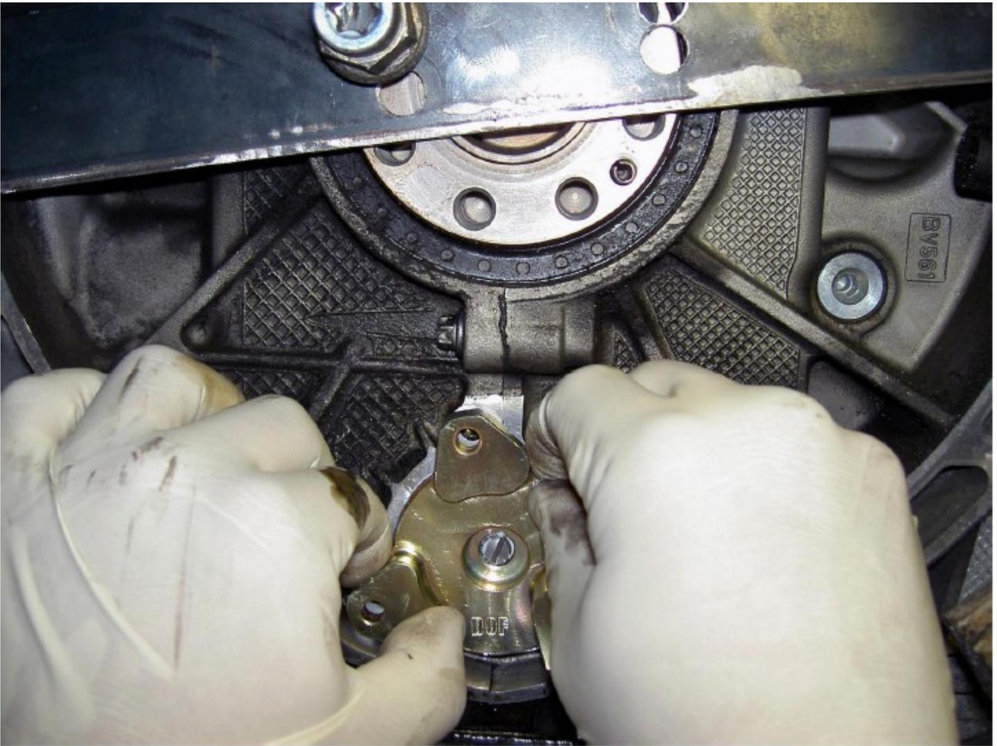
Thread one of the old, removed bolts in place on the top most hole of the flange.
