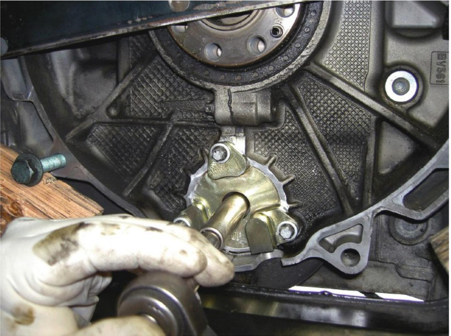
Put a bit of thread locker (supplied) onto the threads of the straight hose adapter on the O-ring side.
