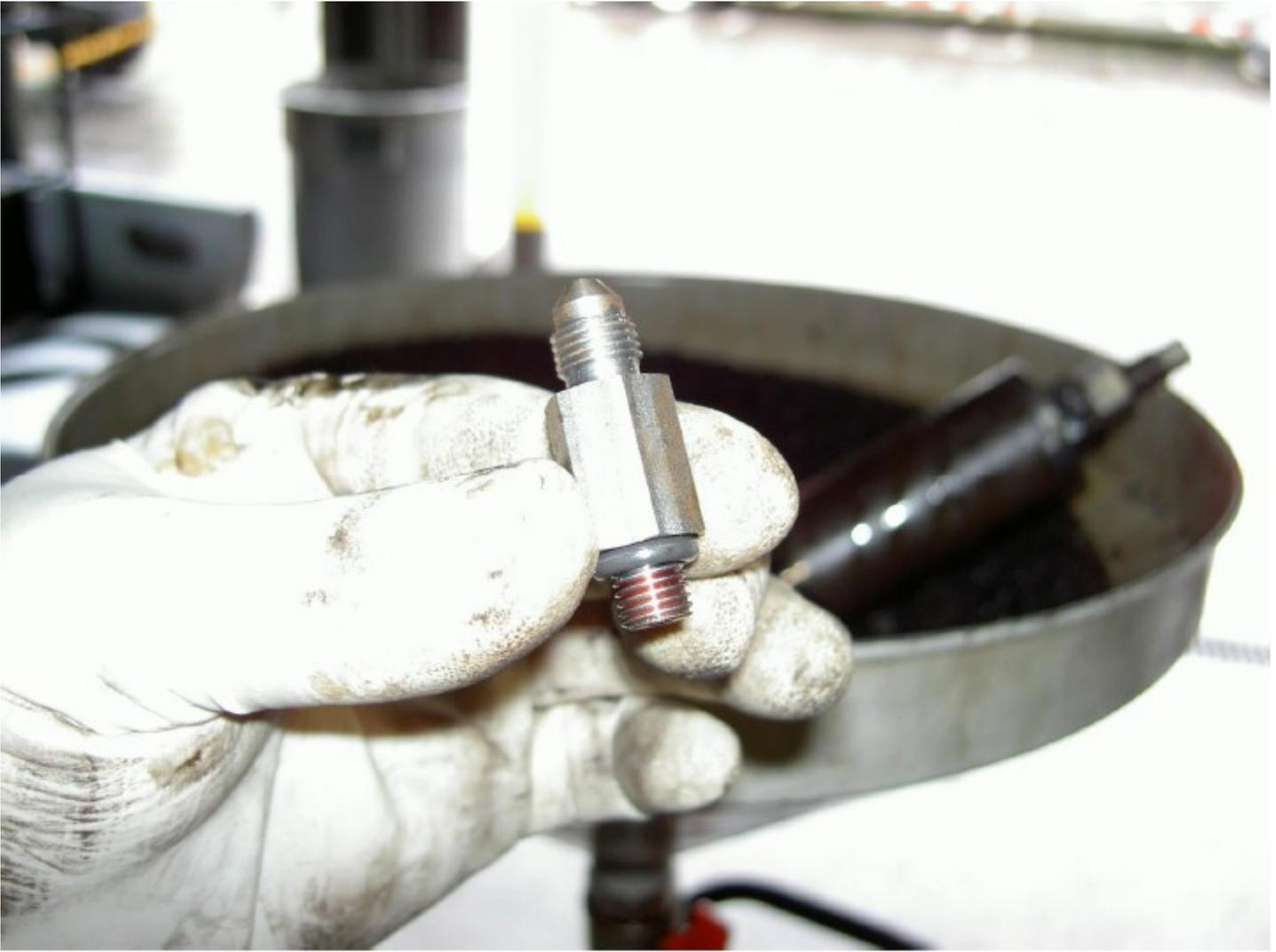
Thread into place onto the DOF flange. Note that the o-ring end of the hose adapter screws into the DOF.
