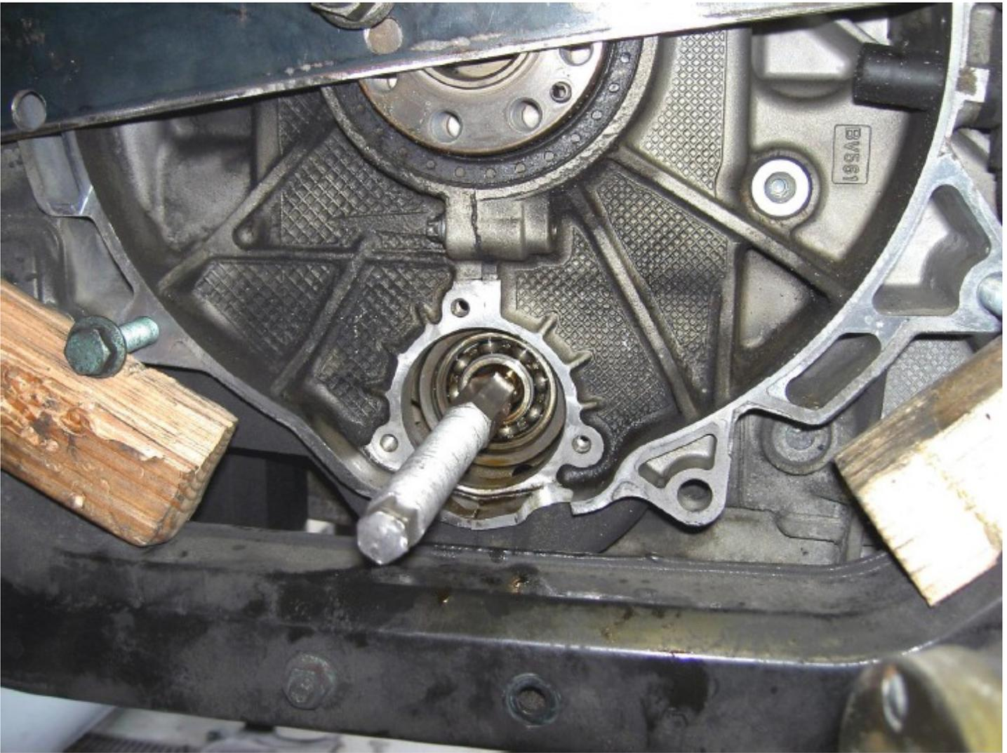
Place the bearing removal tool onto the center bolt and tighten the main nut by hand so that the tool is completely against the engine case.
