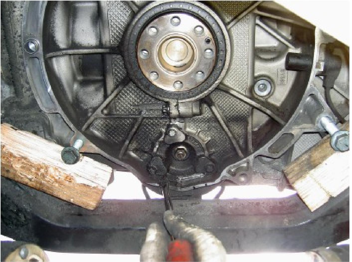
To allow you more working room, on the Boxsters remove the side of the engine's lower safety cable from the engine support yolk immediately under where you will be grinding into the bell housing. On the Carreras, loosen and move out of the way the rear sway bar.
