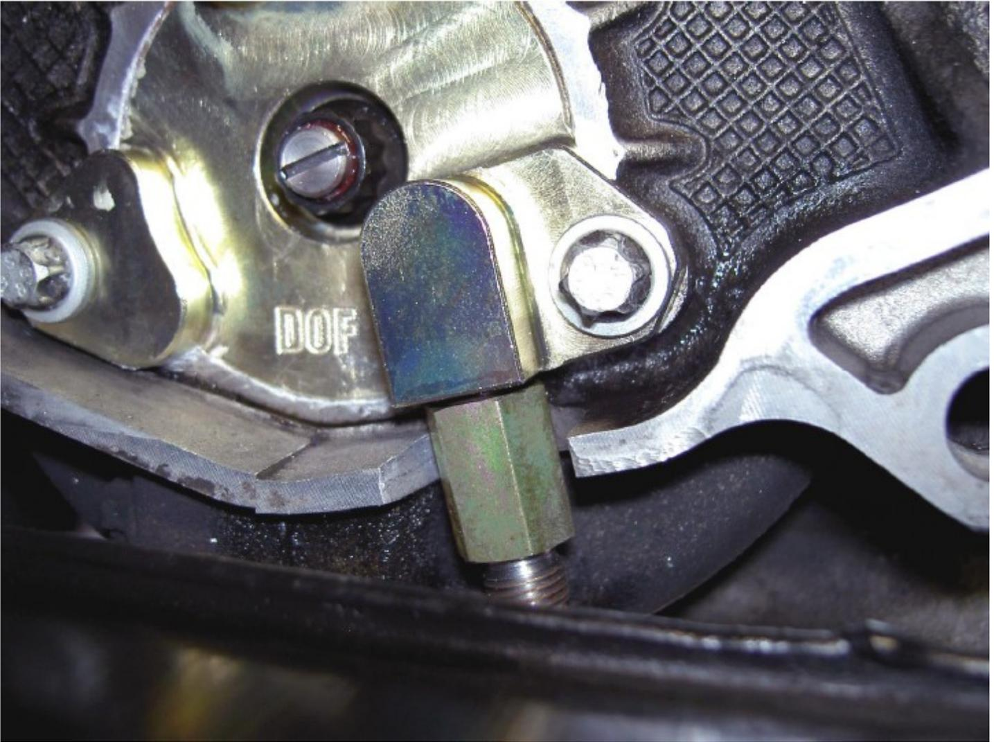
Tighten to a torque of 13 Nm (10 lb-ft or 115 lb-in).
