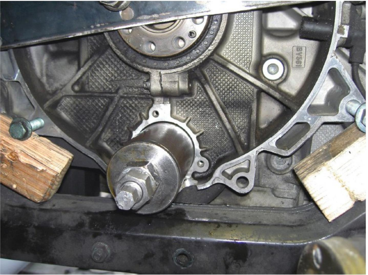
With a wrench, hold the center bolt so it doesn't rotate and start tightening the main nut slowly. At some point you may hear a loud pop which is normal. Keep tightening the main nut until the bearing is completely removed. The bearing will come out inside the removal tool.
