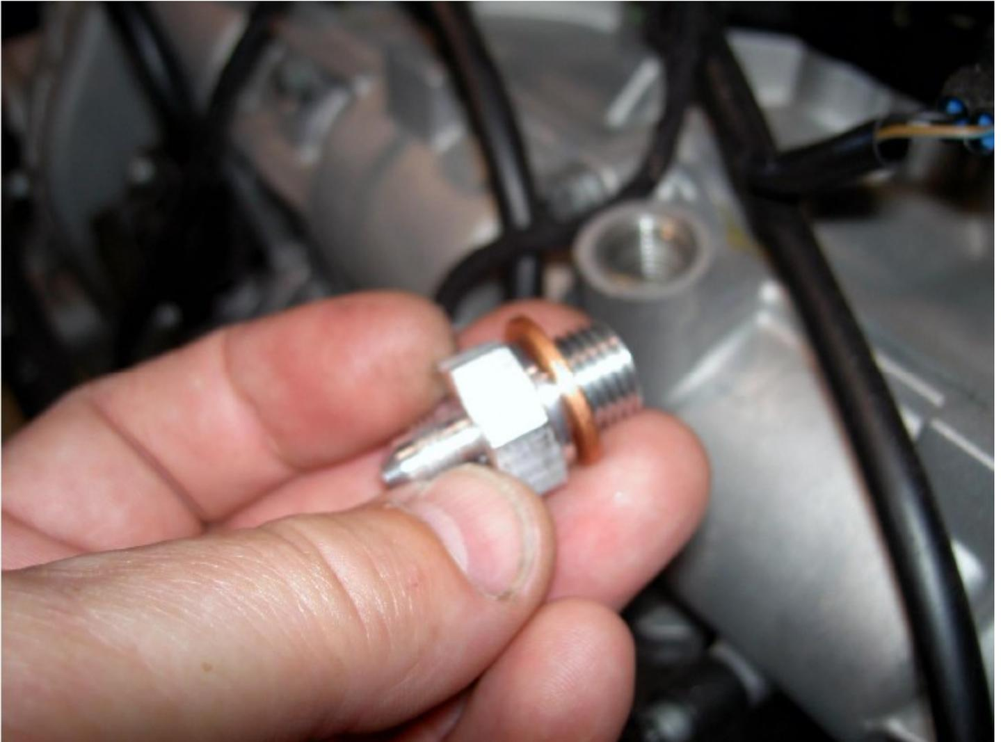
Finally thread the free end of the high pressure oil line onto the newly inserted adapter and torque to 13 Nm (10 lb-ft or 115 lb-in).
