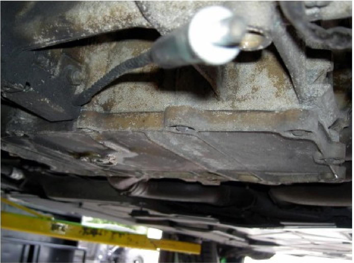
Using an electric or air grinder and correct bit for soft metal and/or a hand saw, cut at the measured marks on the bell housing edge. Cut deep enough to be able to pass and connect the oil line's fitting into the new flange. You can cut all the way through the bell housing nerve up to but not into the engine case.
