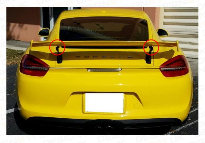
4. The 987C fitment requires the uprights to be mounted on the inner side of spoiler brackets. See the picture below for reference.
