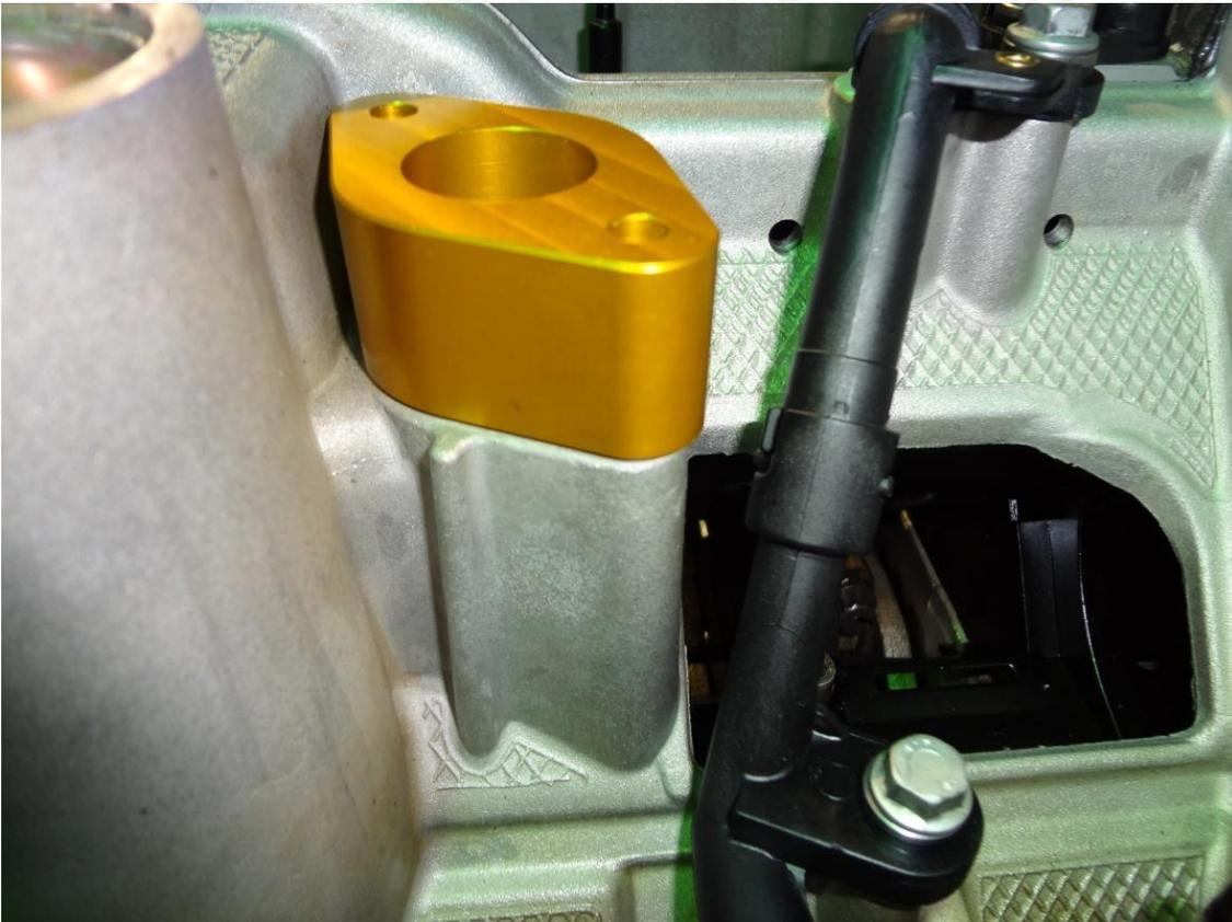
**Step 4:** Install oil pickup return tube and bolt down using two of the supplied hex bolts.
