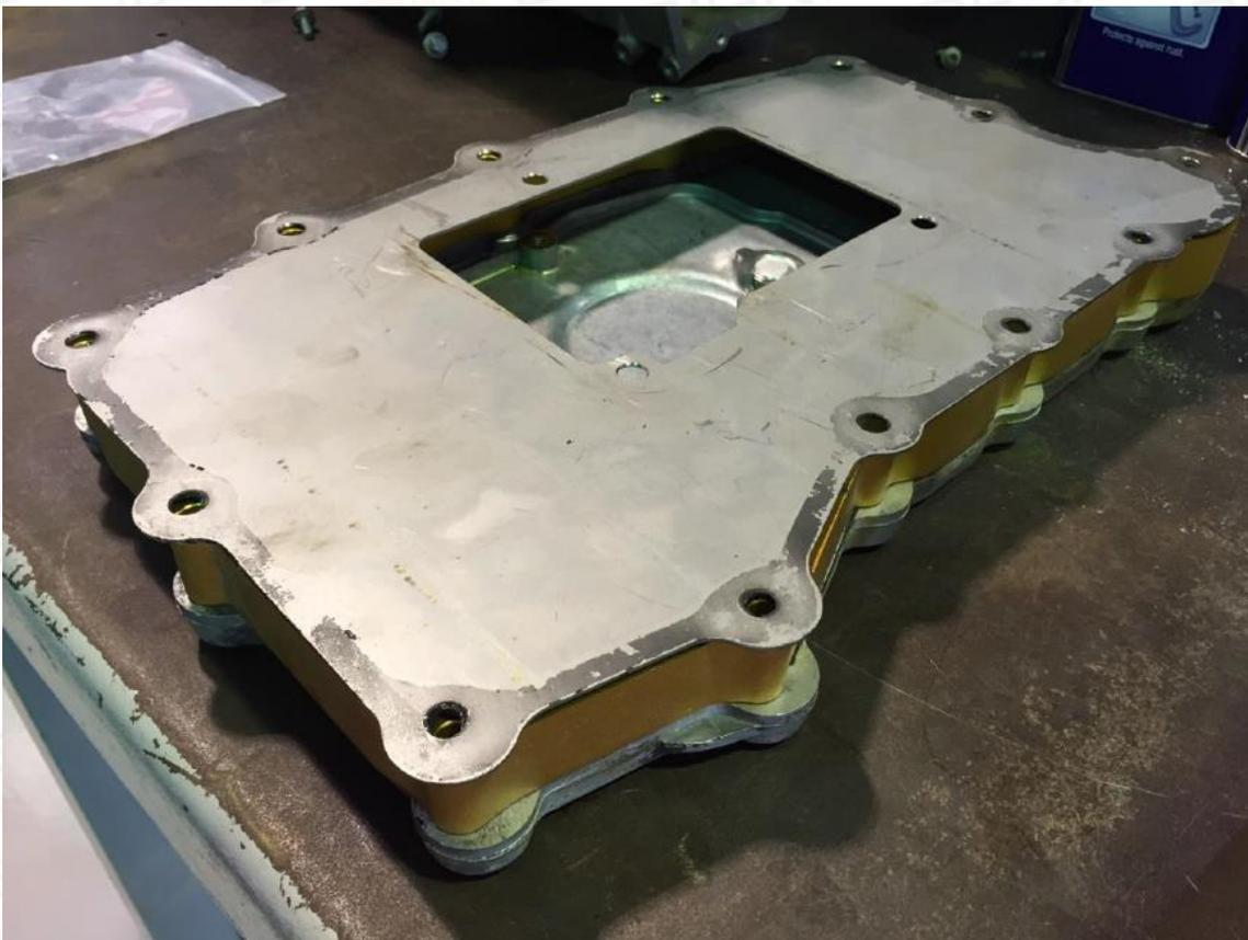
With the baffle in place, align the 3 aluminum 1" spacers between the baffle plate and oil pan.
