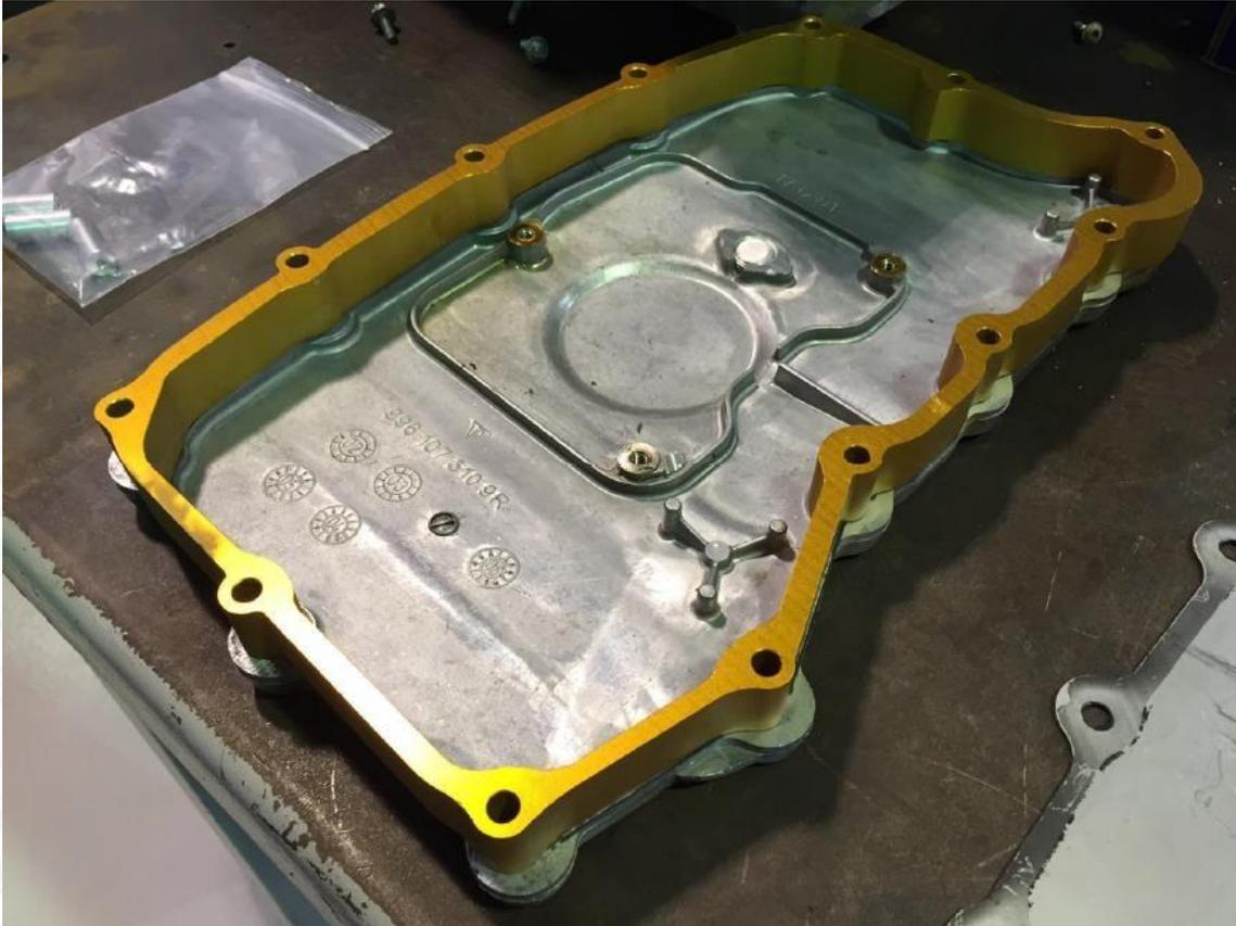
Next, mount the baffle plate to the deep sump extension
