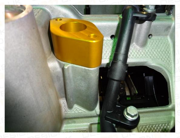
Step 4: Install oil pickup return tube and bolt down using two of the supplied hex bolts.
