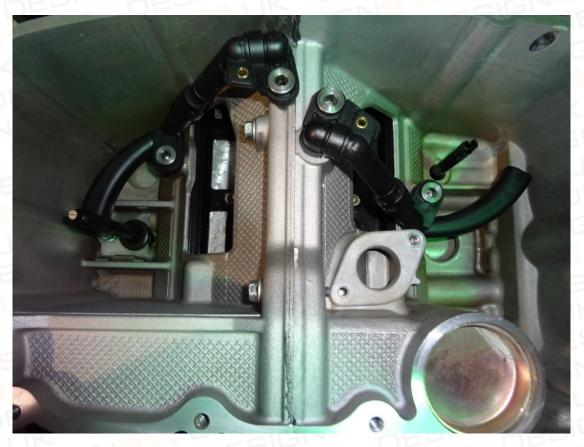
**Step 3:** Install oil pickup tube aluminum spacer as shown below.
