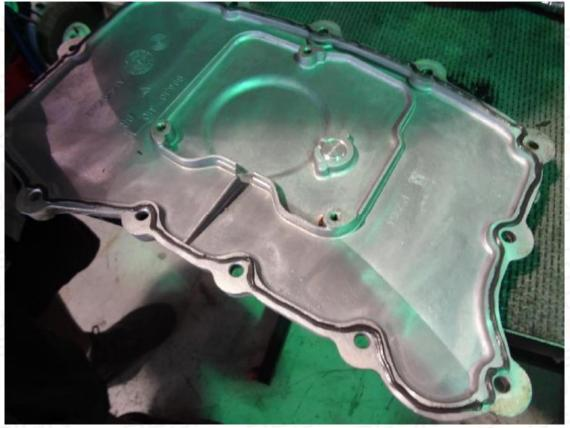
The aluminum baffle spacer does NOT mount to the oil pan itself, it will mount between the engine block and 2 quart extension. The 2 quart extension will mount directly to the oil pan, with the aluminum baffle spacer between block and extension. (see below).
