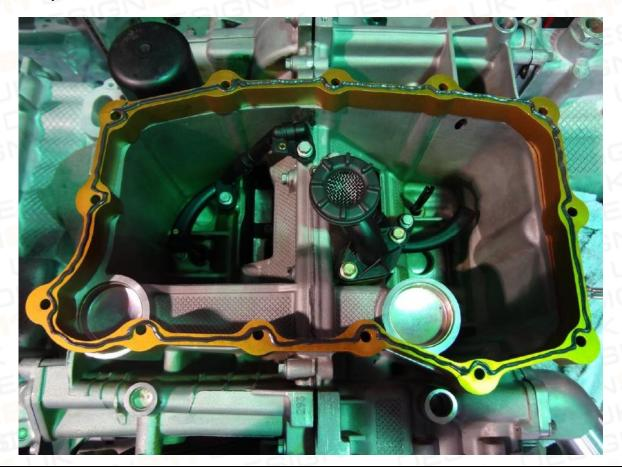
Mount the deep sump extension to the pan. (Note, the photo does not show the pan extension with the sealant. Make sure you have applied the sealant before installing the aluminum baffle on top).
