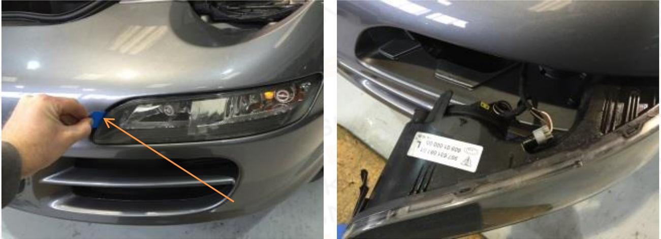
11. Take the green and black wires from light kit and cut to length so long enough to reach from headlamp to bumper lamp. Then tape at various points to make a mini loom.
