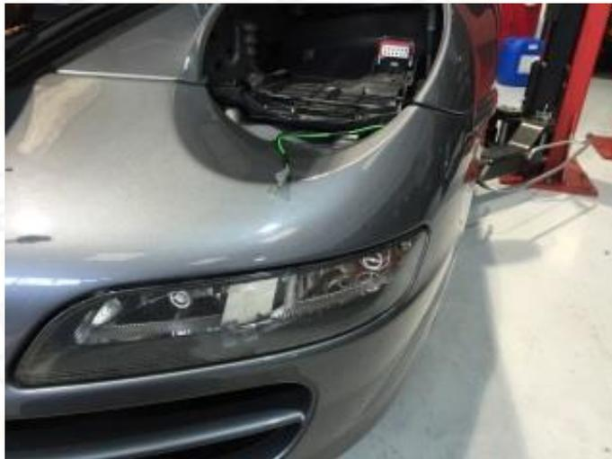
15. Take new lamp and join green wire of mini loom to green loom of headlamp and the same with the black wire.
