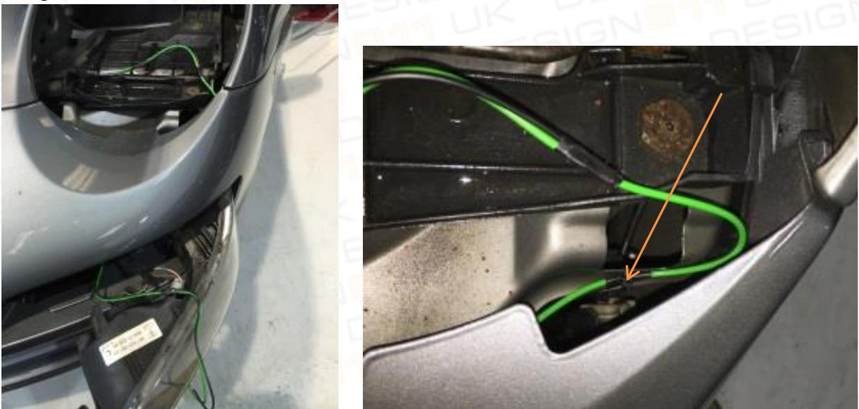
13. Solder green wire on mini loom to white and red on left bumper lamp side light bulb holder and grey and red on right bumper lamp side light bulb holder. Then black wire to brown wires on bumper lamp loom. Then tape to make part of car loom.
