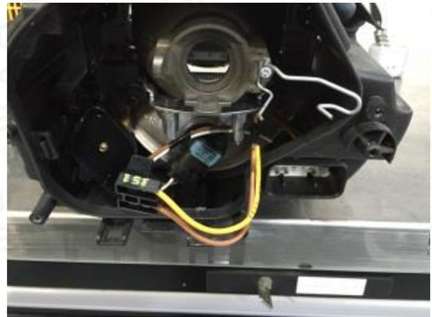
9. Remove 6 screws that hold rear cover on new headlamp then fit bulb. Secure with clip and fit connector.
