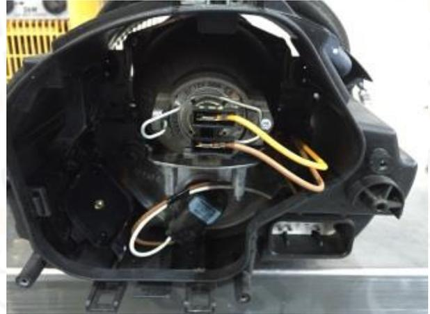
8. Remove Electrical connector and clip that holds bulb then remove (don't touch bulb).
