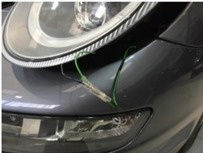
16. Carefully slide the headlamp in to place being careful to tuck any loose wires out of harms way.
