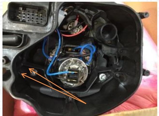
10. With bumper lamp removal tool release front bumper lamps and pull forward.
