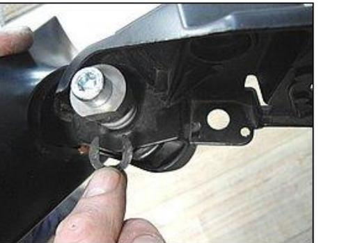
Remove the screw and use the collar to push the snap ring off.
