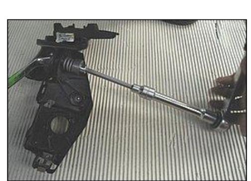
**Compress the spring and remove the U-clamp.**
