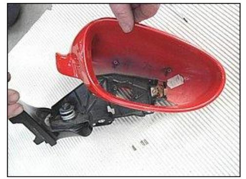
**Insert the screw supplied and tighten the nut.**
