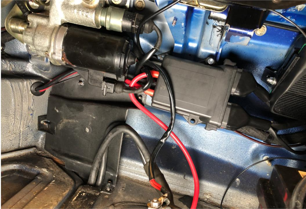
Figure 7 – Hole for heavy red wire, ECU control cable and fan cable on left. ECU can be mounted on front panel.
