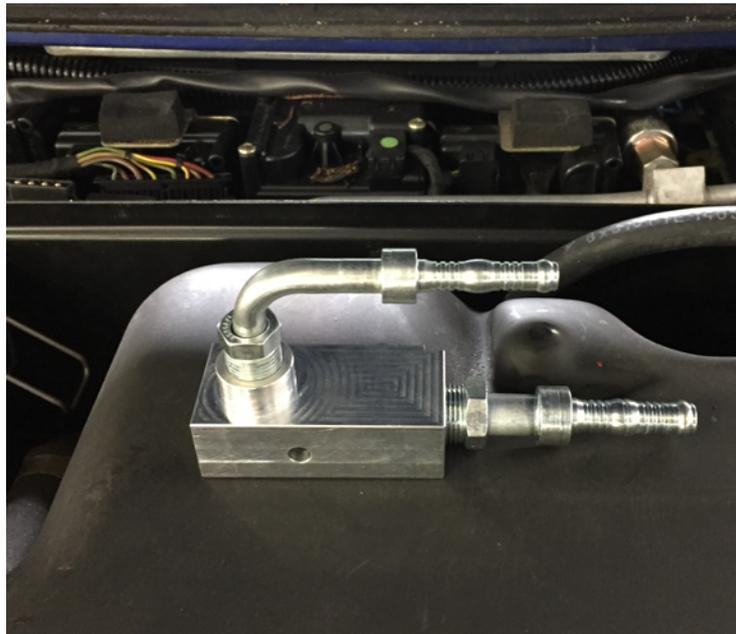
*Figure 1 - Adapter block for flexible hoses.*
