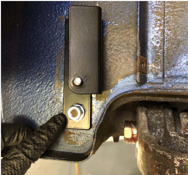
*Figure 10 - Rear condenser mount bracket*
