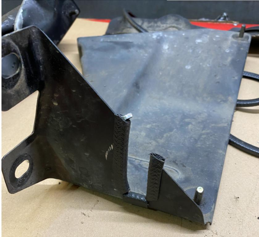
Notch cut in oil cooler support bracket.
