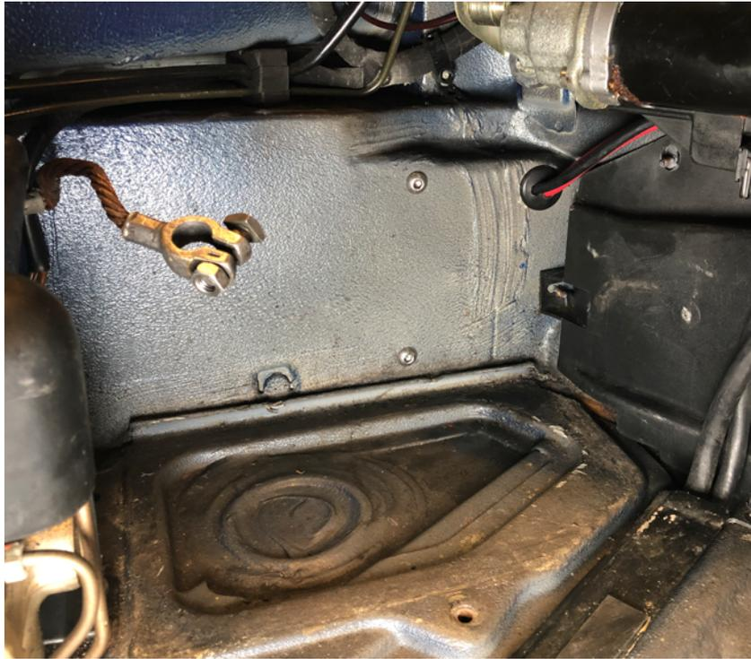
*Figure 4 - Battery side showing 2 x M8 screws. Also note hole on right with grommet for wiring.*
