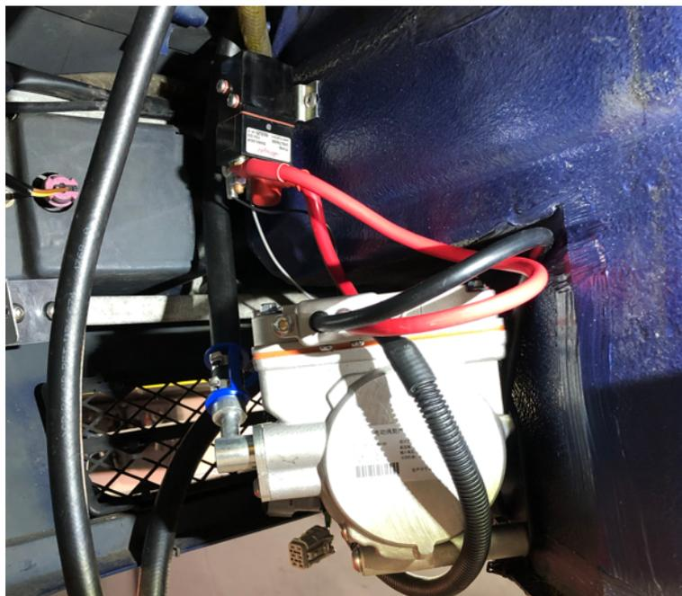
*Figure 9 - Install using isolating contactor relay*
