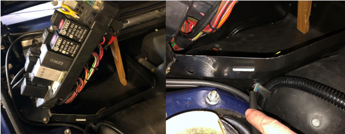
Figure 16 - Feeding Electrocooler loom into front of fusebox.
