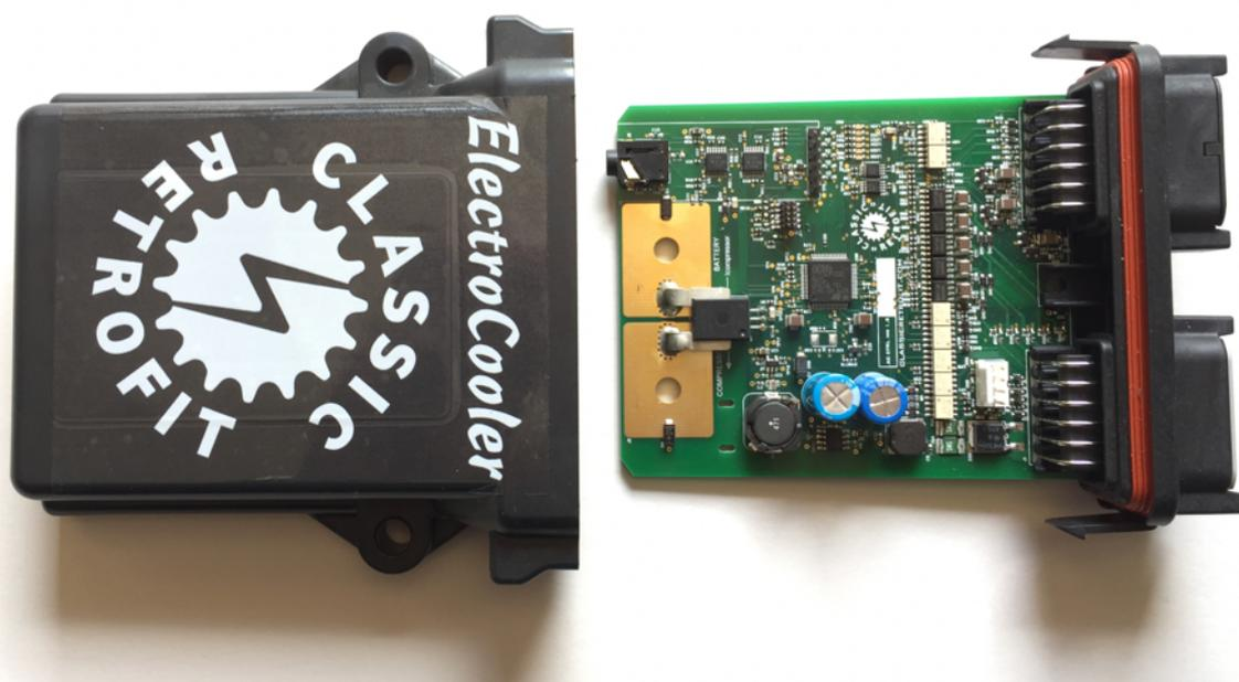
The ECU comes preset with conservative working parameters. It is possible to adjust the values using a laptop as described in our setup manual. It is strongly recommended NOT to adjust these values without reading the manual or consulting us first.
