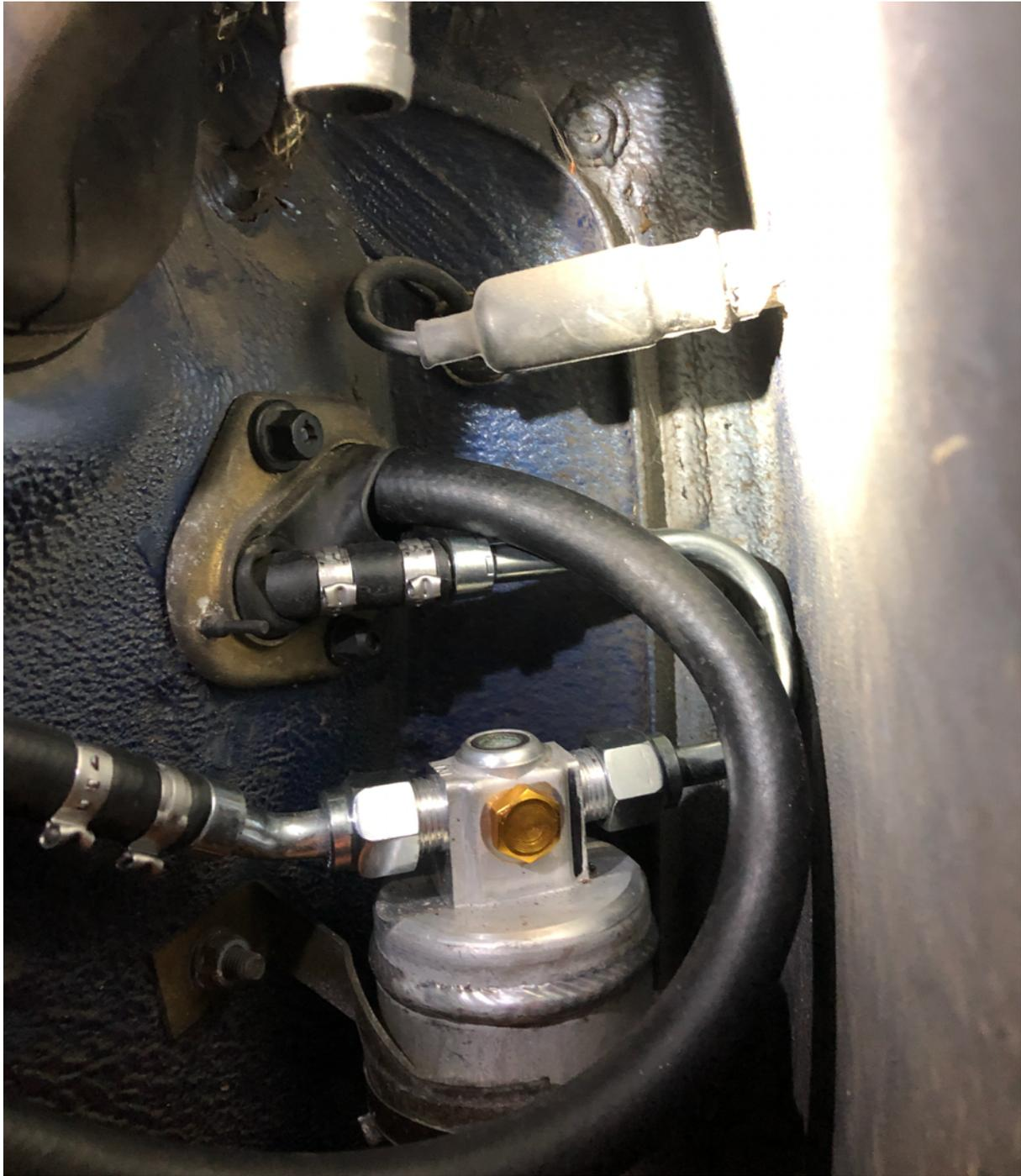
*Figure 14 - Drier can be fitted in standard location.*
