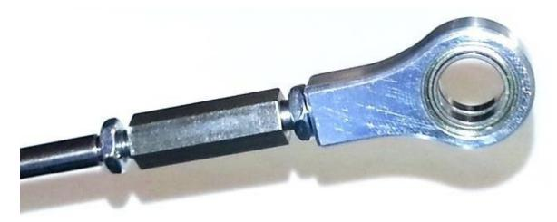
Adjustment will move shift lever position. Be sure to have it's in the desired position before securing.
