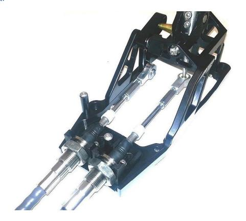
When installing the cables components make sure to apply the plastic caps to all ball end mounts.
